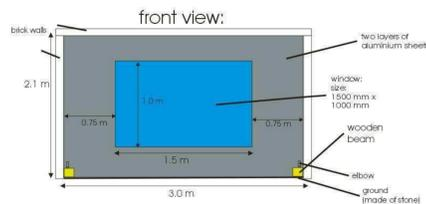
FIGURE 1: Wall construction and dimensions to test both standard and low emissivity window types.
