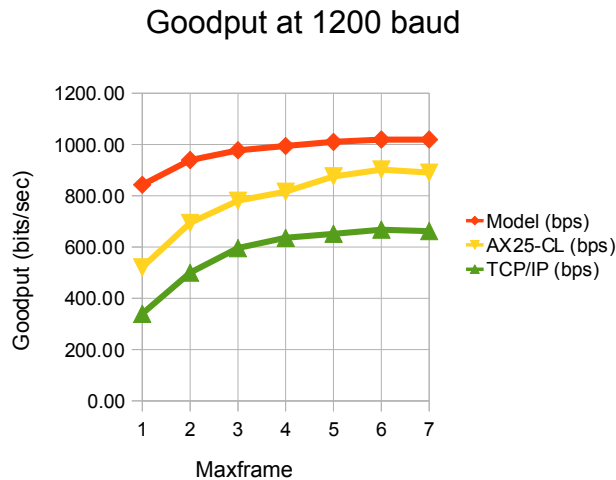
Fig. 4. Comparison of transfer times for AX.25CM-CL and TCP/AX.25 with reference to theoretical model at 1200bps.
