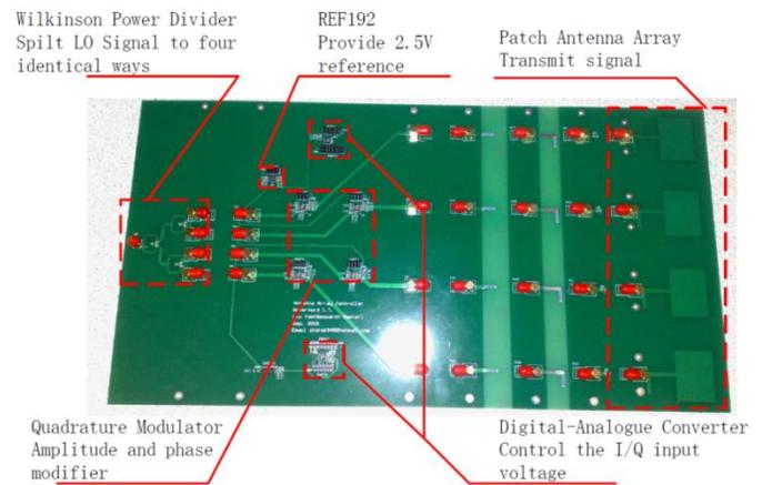
Fig. 2 Complete PCB fabrication (pre-separation)
