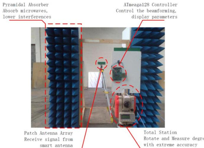
Fig. 3 Picture of antenna gain test set-up
