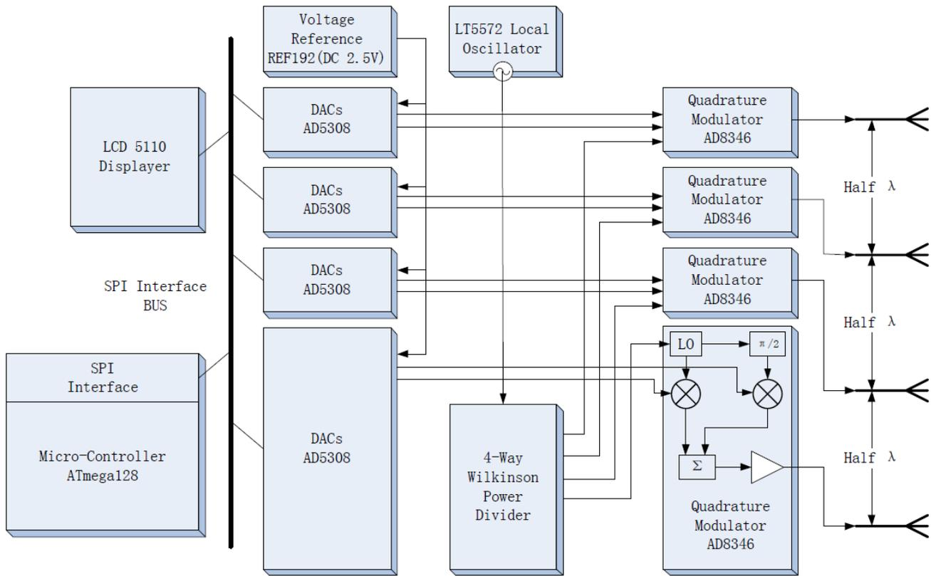
Fig. 1 Block diagram of test system
