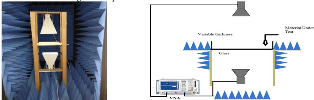
Figure 3 Candidate vertical measurement systems, in WIT anechoic chamber
