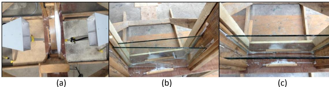
Figure 1: Issues with container rigidity and misalignment
