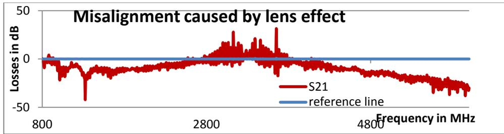
Figure2: Misalignment of a salt measurement result caused by lens effect
