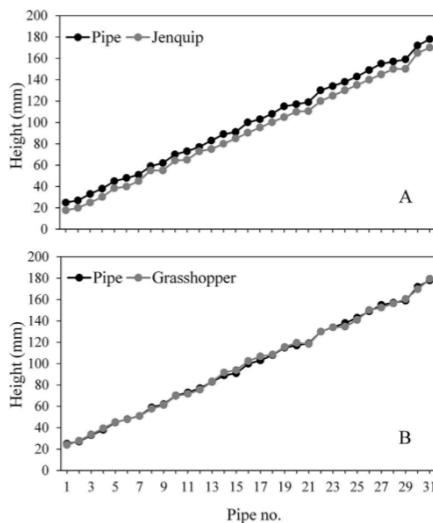
**Fig. 2 – Comparable ability of the cumulative ratchet counter Rising Plate Metre (A: Jenquip), and micro-sonic sensor Rising Plate Metre (B: Grasshopper), to accurately measure fixed heights ( $n = 31$ ). Standard error  $\leq 1$  in all cases.**
