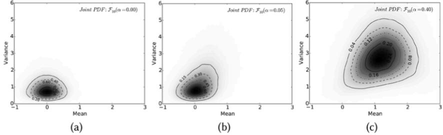
Fig. 3. Gaussian Mixture Effect on joint windowed mean and variance distribution. (a) No effect ( $\alpha = 0.0$ )
