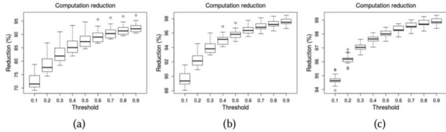
Fig. 17. Effect of  $\varepsilon$  on reduction of IEM classifications for  $windowSize$  (a) 10s (b) 30s (c) 60s.
