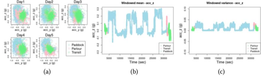
Fig. 12. (a) Acceleration of a cow during different activity states in the  $y$ - $z$  plane (b) Windowed mean of  $acc_z$  (c) Windowed variance of  $acc_z$  at  $windowSize = 60$ .
