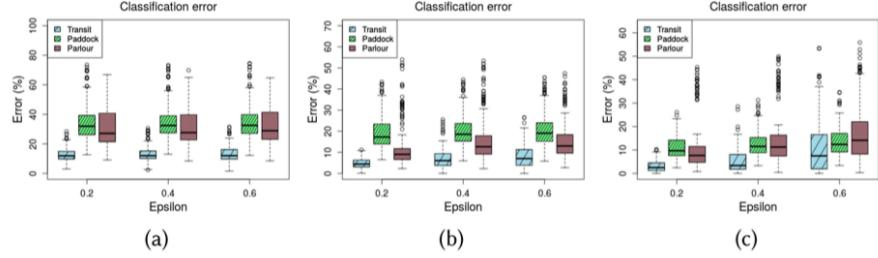
Fig. 18. Effect of  $\epsilon$  on classification error of IEM for  $windowSize$  (a) 10s (b) 30s (c) 60s.
