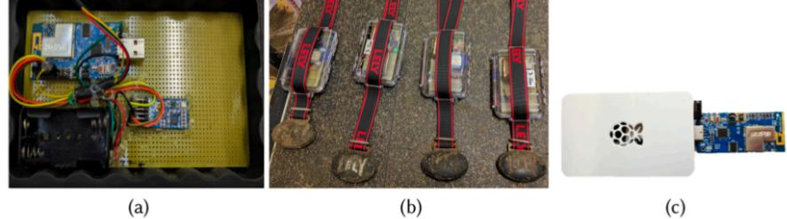
Fig. 8. (a) and (b) Animal-wearable collar devices (c) Cloud gateway.
