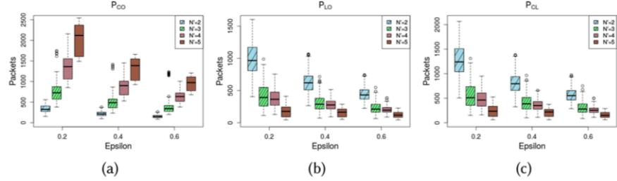
Fig. 22. Effect of coalition size on (a)  $P_{CO}$  (b)  $P_{LO}$  (c)  $P_{CL}$  at  $windowSize = 60$ .
