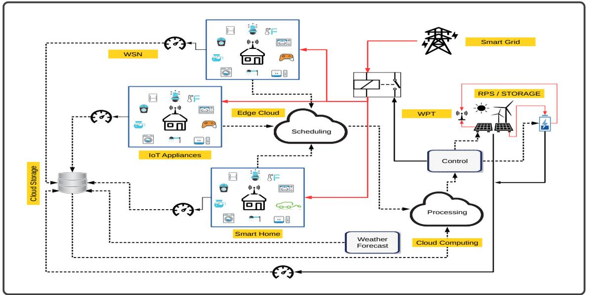
Figure 3: Topology of the wIshood's architecture. It is formed by the scheduling, information, communication, processing and control layers. The RPS supplies energy to the households using WPT technology.
