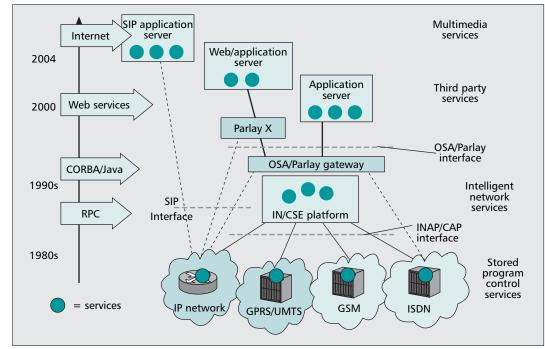
**Figure 1**. Evolution and relationships between different service delivery platforms.
