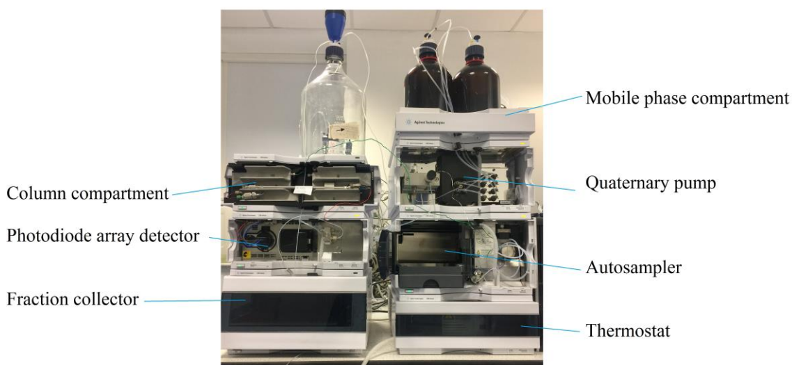
Figure 2.4: Instrumentation of a high performance liquid chromatography (HPLC).
