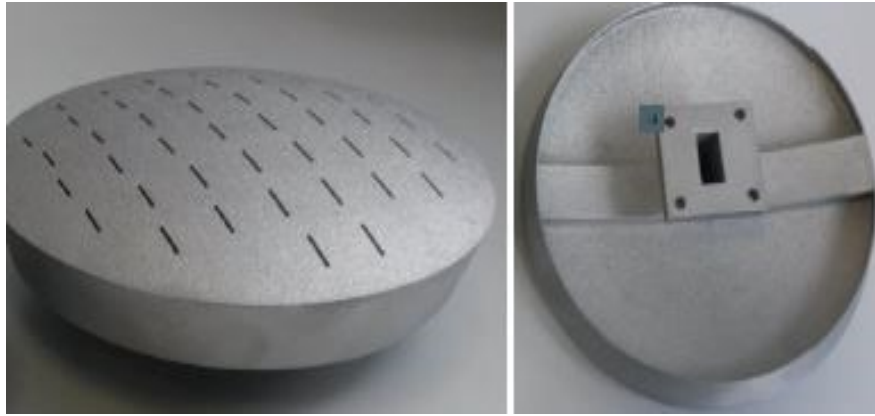
Figure 8: 3D Conformal slotted waveguide antenna array [41]
