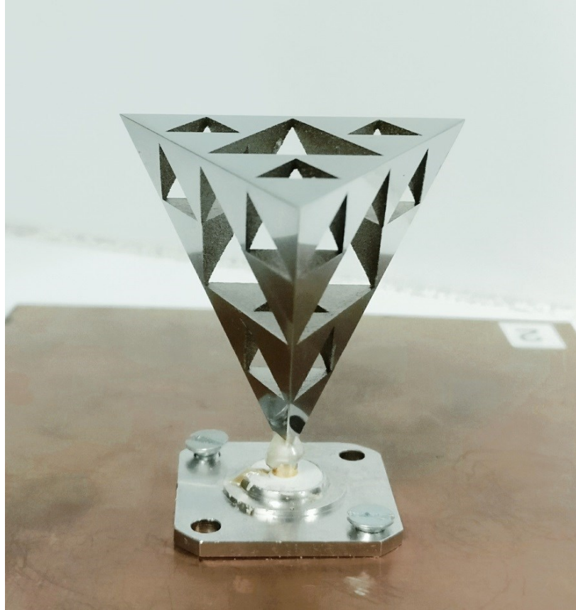
Figure 38: Sierpinski gasket antenna after polishing
