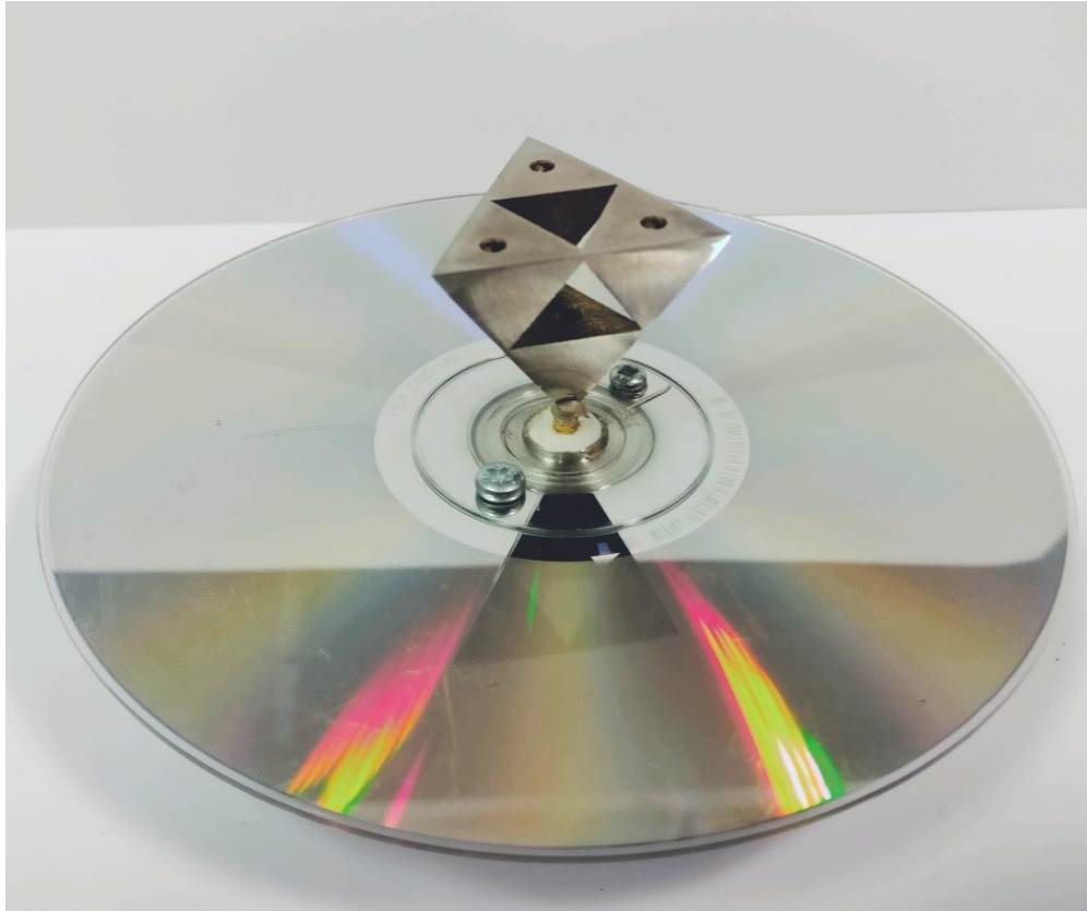
Figure 55: 3D metal printed inner lattice antenna with CD as ground plane
