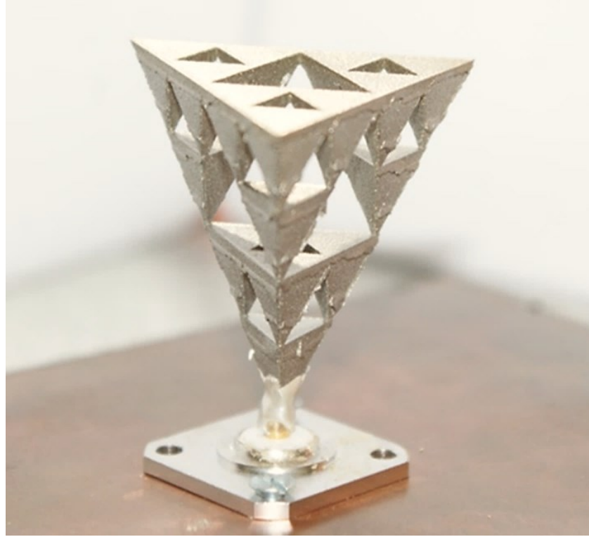
Figure 35: Sierpinski gasket antenna fabricated after wet blasting
