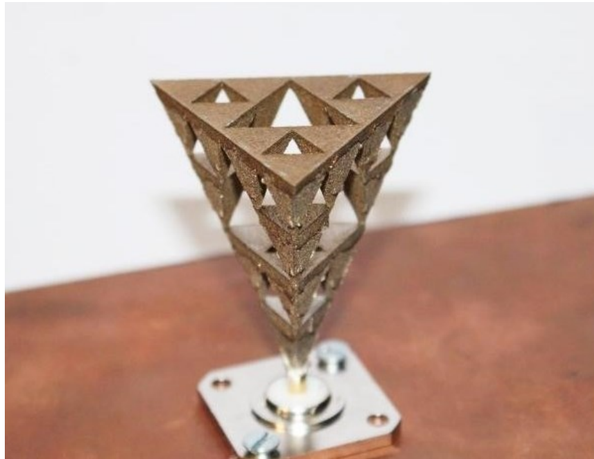
Figure 32: 3D metal printed Sierpinski gasket antenna, after heat treatment
