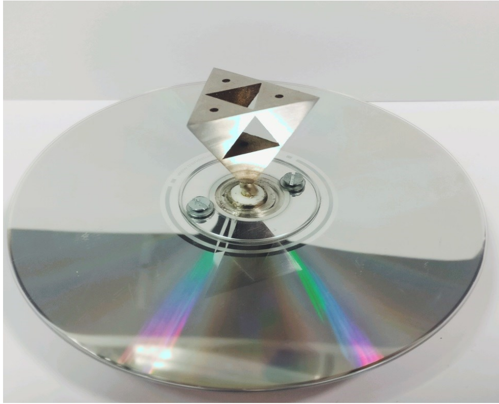
Figure 54: 3D metal printed hollow antenna with CD as ground plane
