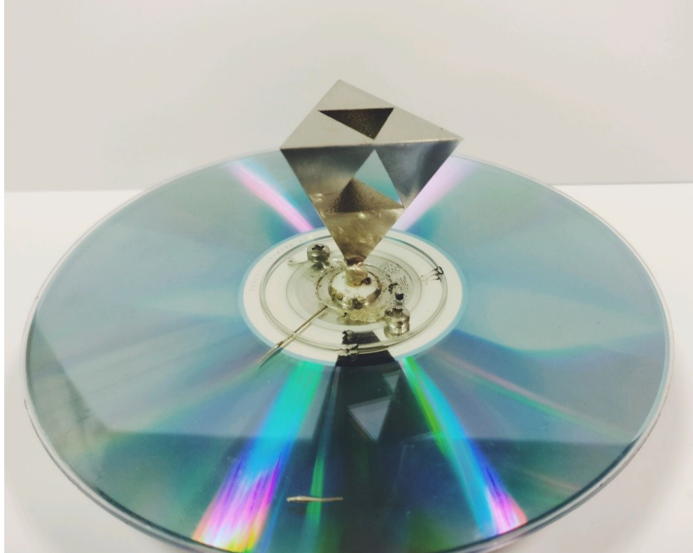
Figure 51: 3D metal printed solid antenna with CD as ground plane
