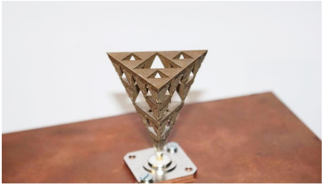
Figure 10: Sierpinski gasket antenna fabricated using DMLS technology on Ti-6Al-4V
