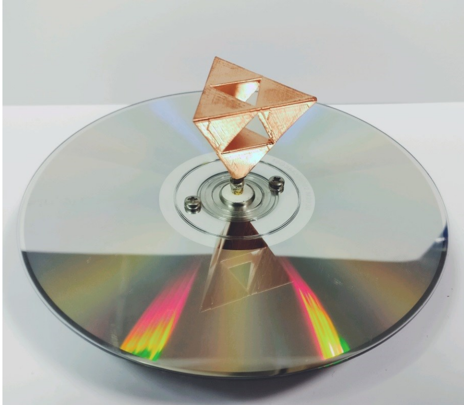
Figure 57: 3D metal-coated polymer printed antenna with CD as ground plane
