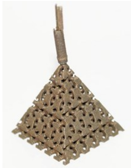
Figure 43: Experimental prototype and monocone antenna with an integrated feed
