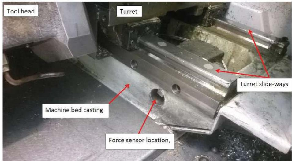
**Figure 23** Force sensor location in relation to slideways and turret
