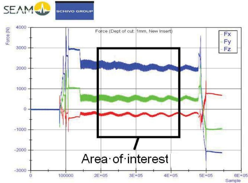
**Figure 59** Force sensor results for each axis, 1mm cut, and area of interest
