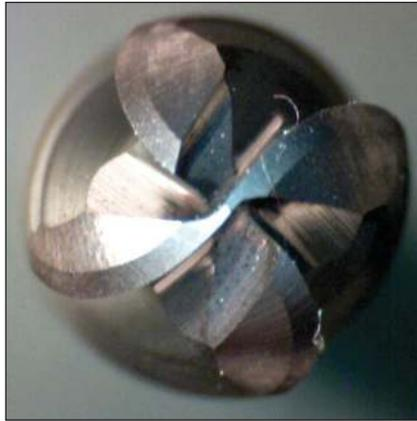
**Figure 39** New tool- front view 50X
