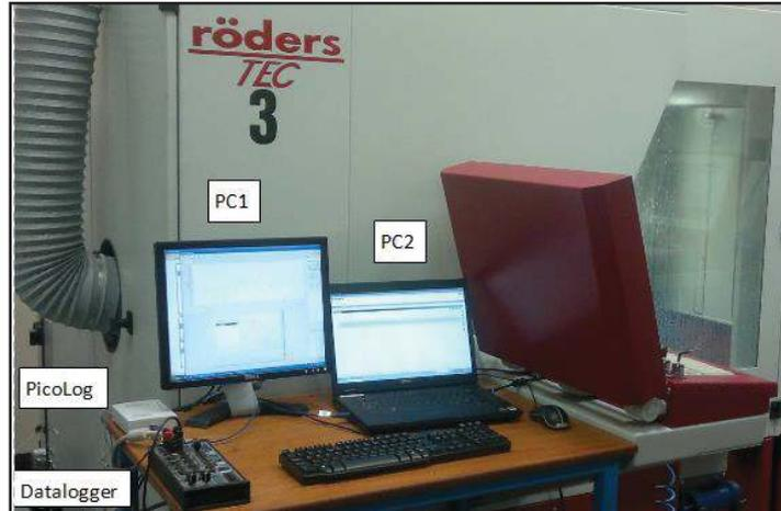
**Figure 15** Overview of PC & datalogger configuration
