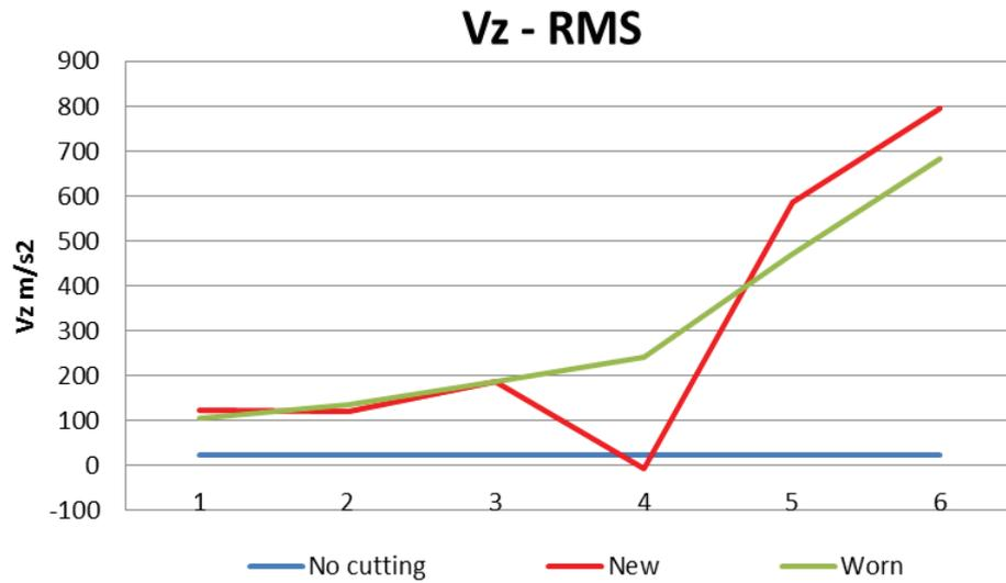
**Figure 65** Sensor Z-axis vibration for depths 1-6mm
