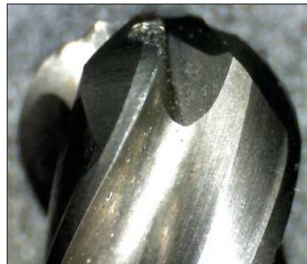
**Figure 42** Worn tool- side view 50X
