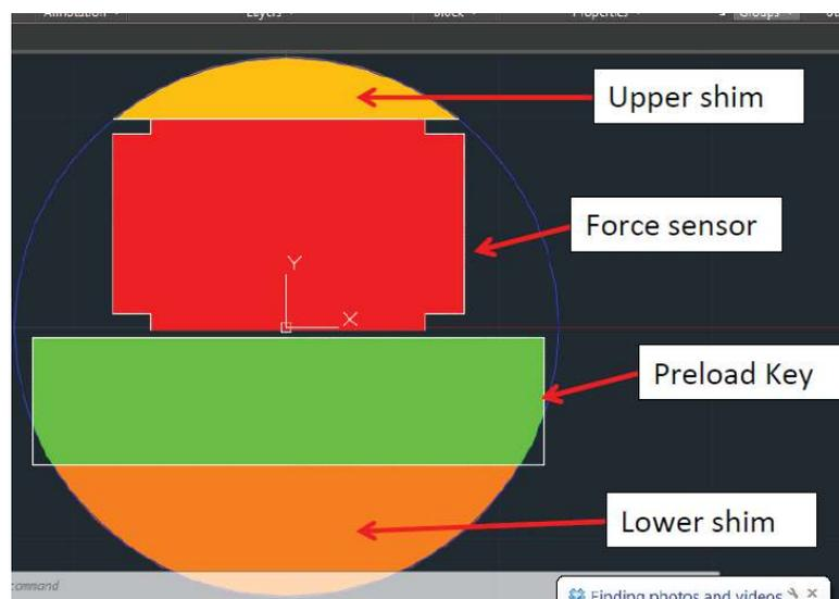
**Figure 24** Sensor/preload key/shim configuration in drilled hole in casting
