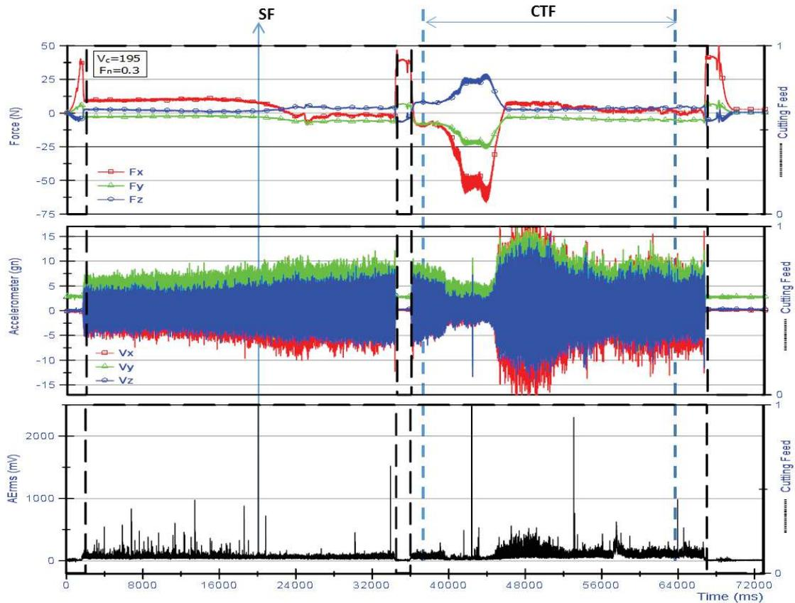
**Figure 69** Sensor signals from CTF instance 3
