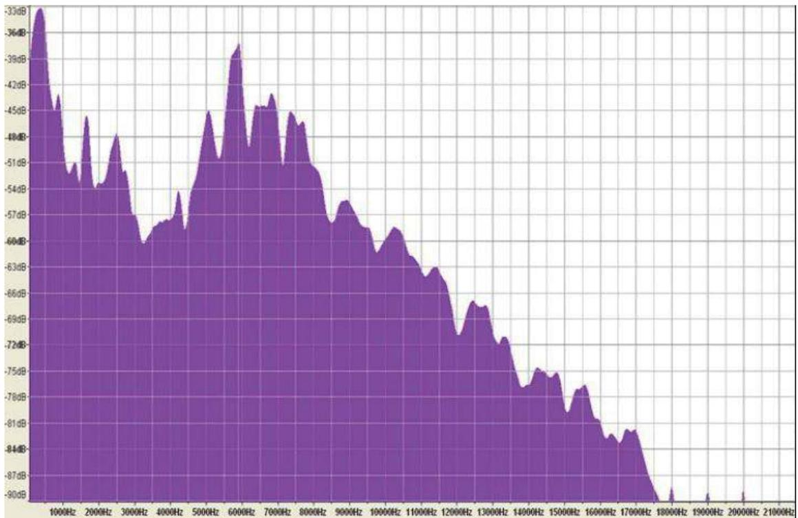
**Figure 9** Frequency domain representation of a Harrison lathe audio signal
