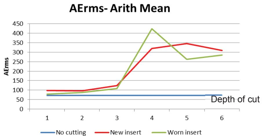
**Figure 66** Comparison of the AE sensor readings for each of the facing passes
