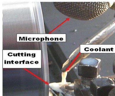
**Figure 5** Microphone configuration
