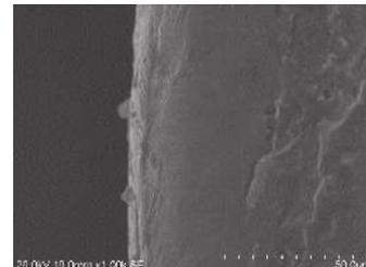
**Figure 32** Worn interface, Trial 2
