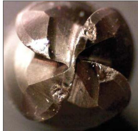
**Figure 40** Worn tool- front view 50X
