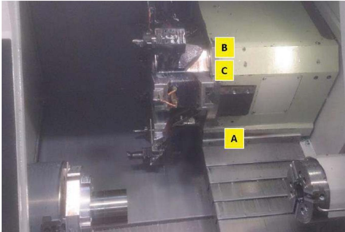
**Figure 21** Sensor locations on the Nexus 200
