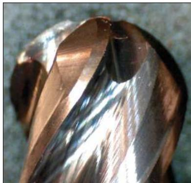
**Figure 41** New tool- side view 50X
