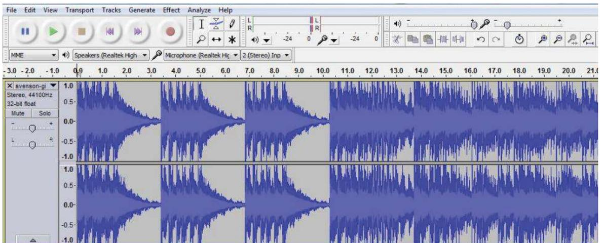
**Figure 8** Typical time domain capture of the Harrison Lathe audio signal
