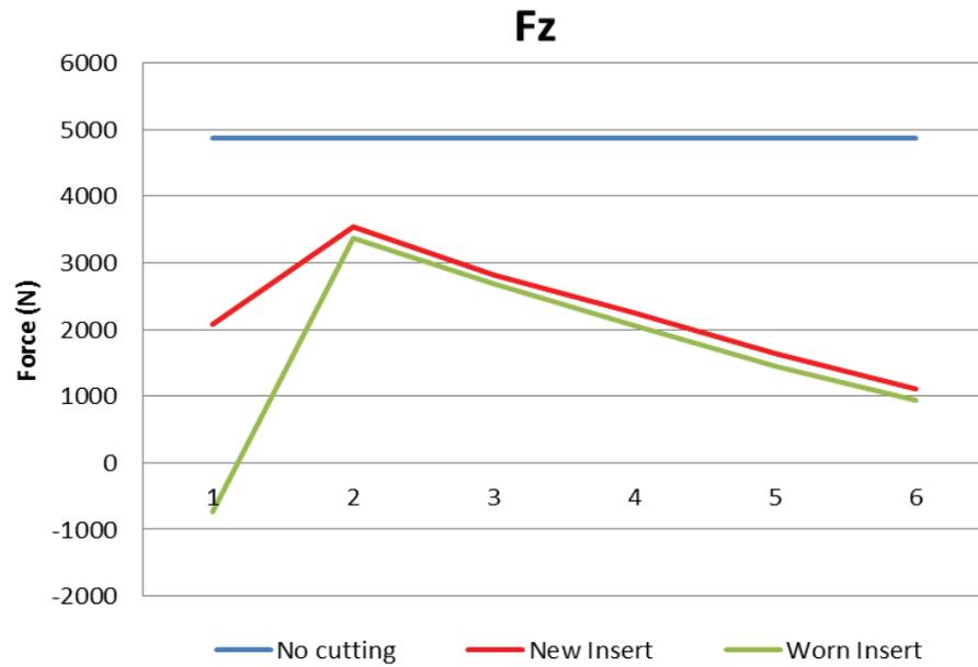
**Figure 62** Sensor Z-axis force for depths 1-6mm
