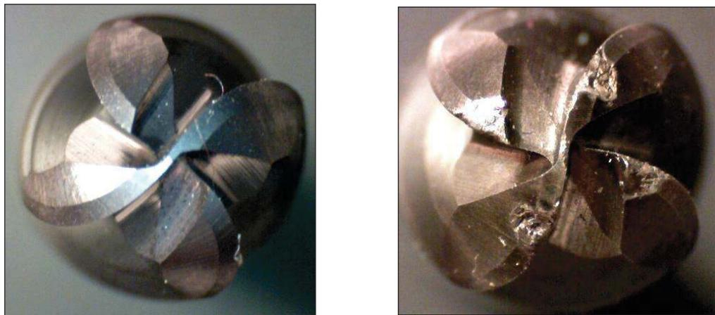
**Figure 16** Photos of new and exhausted ballnose cutter X50 Magnification
