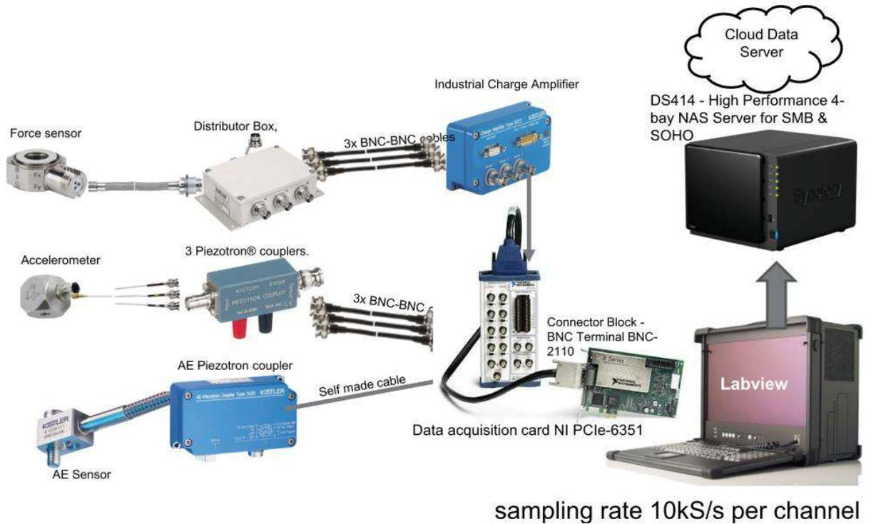
**Figure 19** Outline of configurations for Mazak experiment
