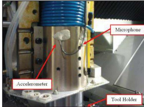
**Figure 12** Sensor locations on machine spindle
