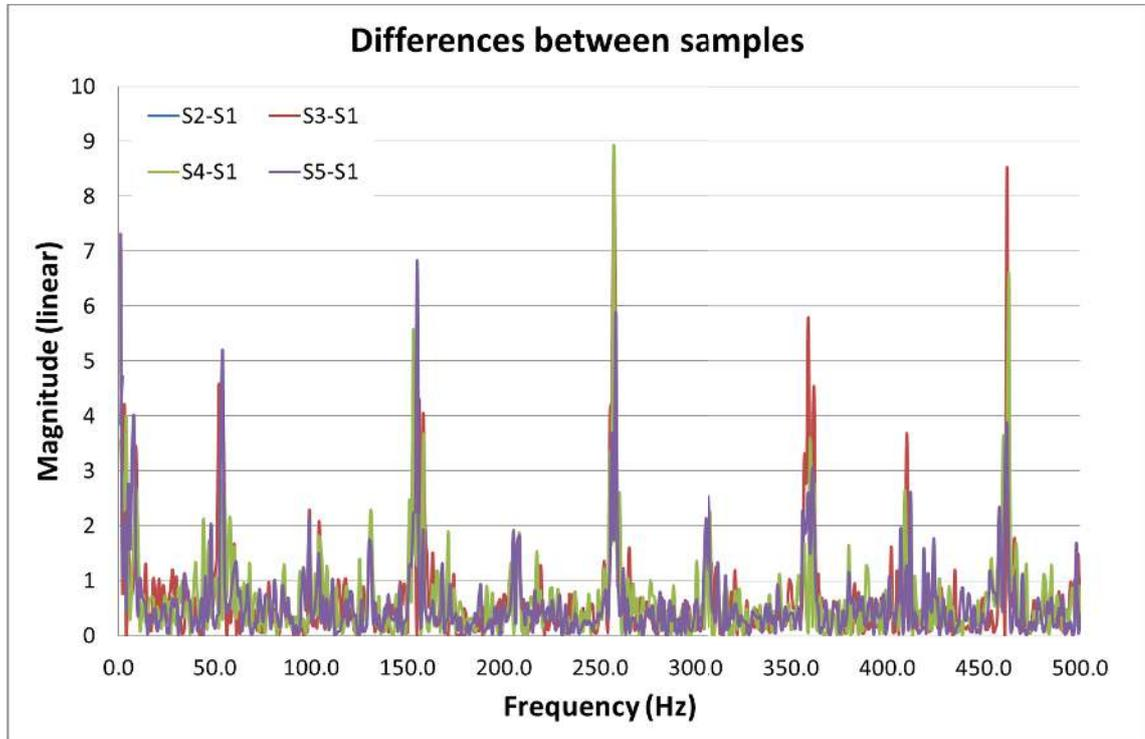
**Figure 58** Frequency domain differences between samples' vibration data
