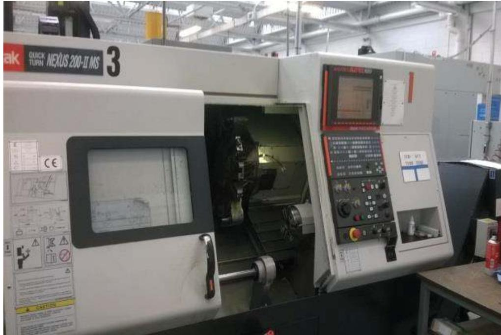
**Figure 18** The Mazak Quick Turn Nexus 200
