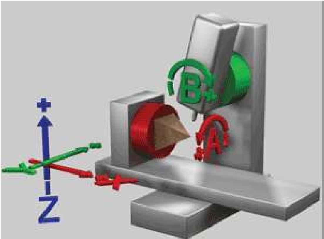
**Figure 70** Illustration of axes in CNC turning
