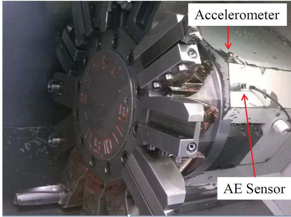
**Figure 22** Accelerometer and AE sensors in relation to the Mazak tools
