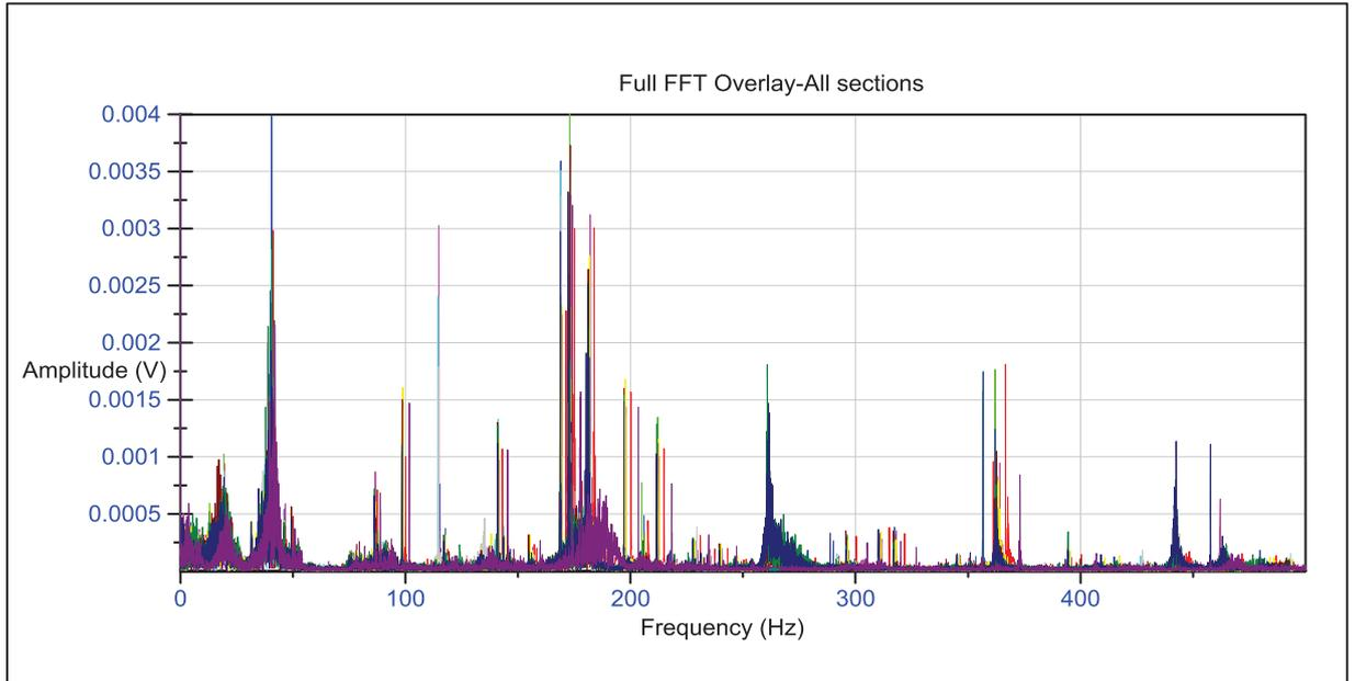
**Figure 46** Full FFT spectrum overlay of all sections (vibration sensor 1).
