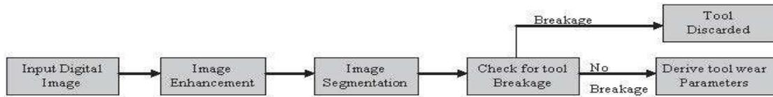
**Figure 2** Block diagram of vision system for tool wear
