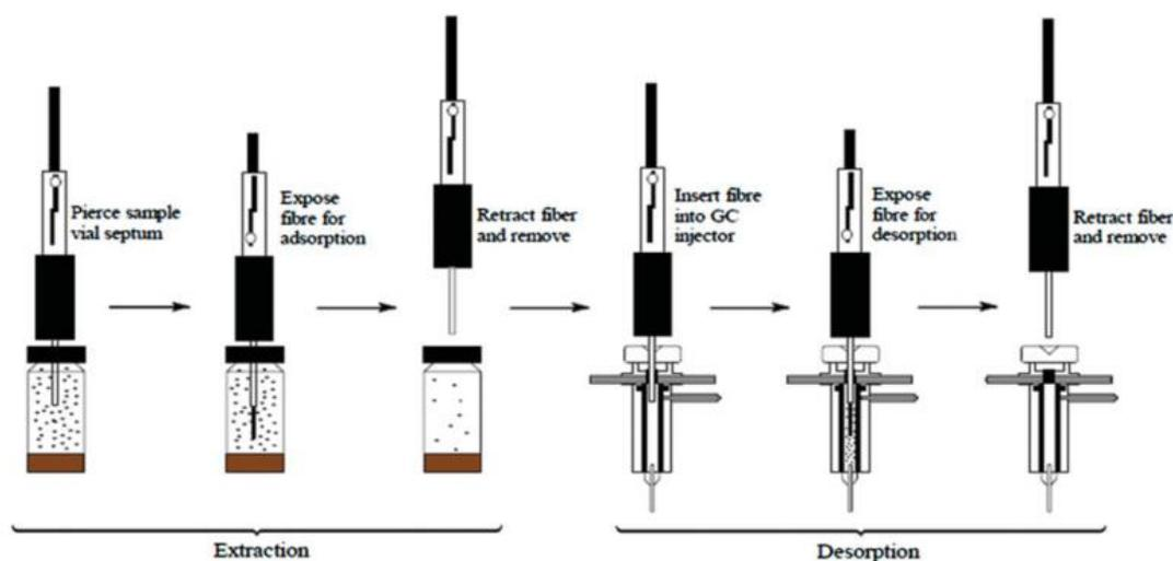
**Figure 1.1:** Schematic of headspace SPME [12].
