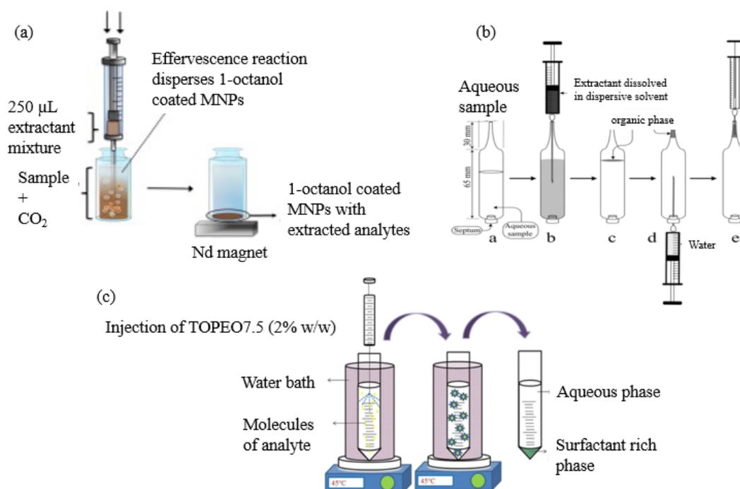
**Figure 1.3:** Schematic diagram of: (a) effervescence DLLME [24] (b) LDS-DLLME using specialist glassware [18] (c) CP-DLLME [28]: Schematic diagram of: (a) effervescence DLLME [24] (b) LDS-DLLME using specialist glassware [18] (c) CP-DLLME [28].
