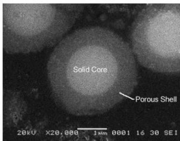
**Figure 2.2:** Superficially porous particle showing the solid core with stationary phase bonded to the surface [87].
