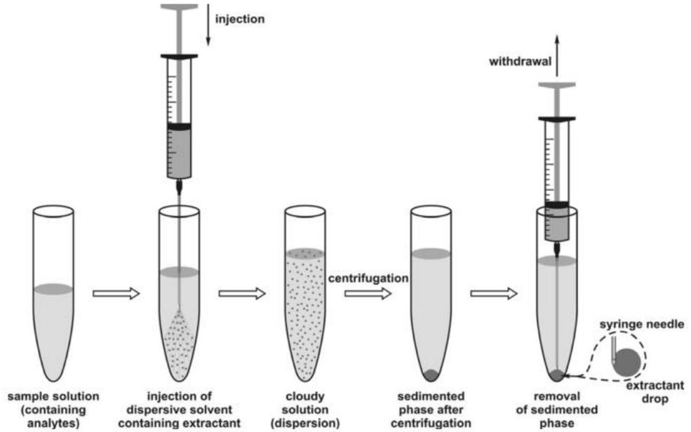
**Figure 1.2:** Schematic of DLLME technique [11].
