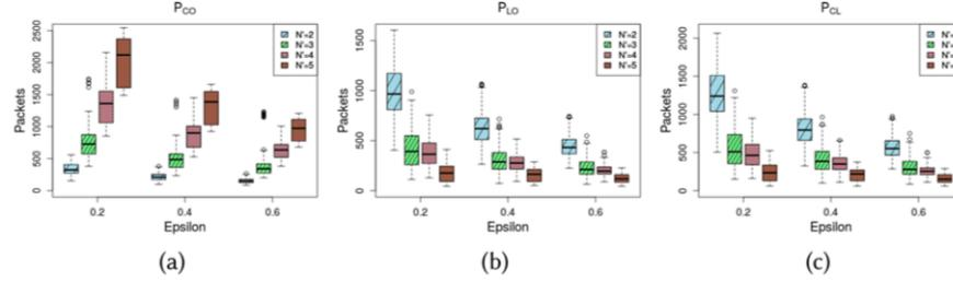
Fig. 22. Effect of coalition size on (a)  $P_{CO}$  (b)  $P_{LO}$  (c)  $P_{CL}$  at  $windowSize = 60$ .
