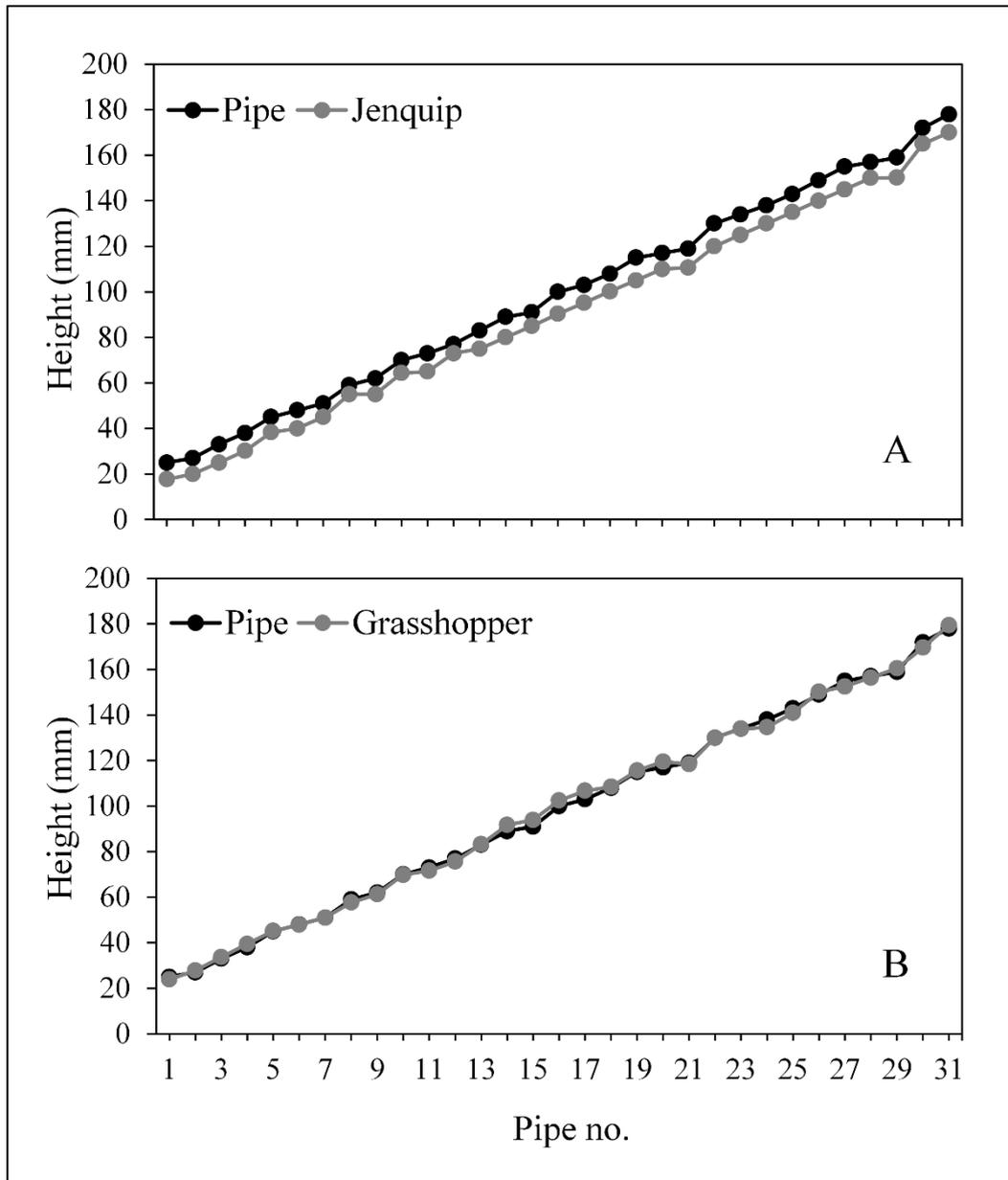
*Figure 3.2: Comparable ability of the cumulative ratchet counter Rising Plate Metre (A: Jenquip), and micro-sonic sensor Rising Plate Metre (B: Grasshopper), to accurately measure fixed heights (n = 31). Standard error  $\leq 1$  in all cases.*
