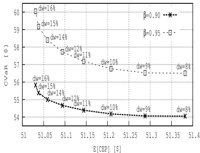
Fig. 3.5 Efficient frontier for different  $d_w$ .  $\alpha = 0.7$  and two worst case scenarios.
