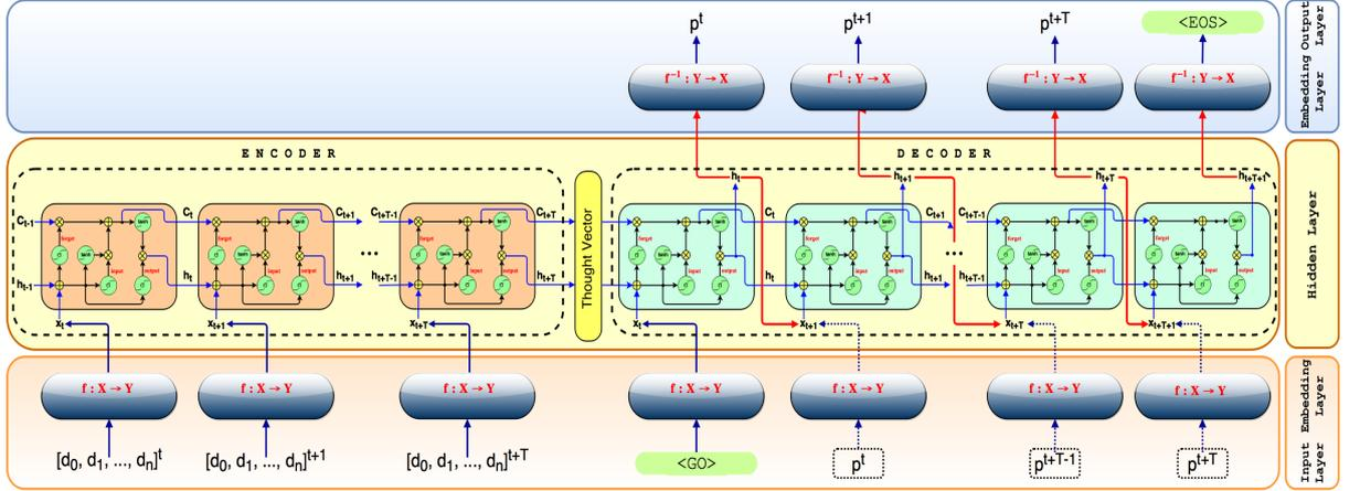
Figure 4: The architecture of the DS2S prediction instance are three main layers: Input, Hidden and Output. And the ancillary Embedding layers. The Hidden layer consists of stacked LSTM cells.
