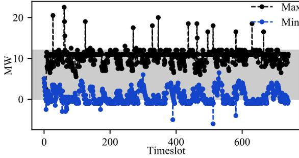
Figure 5: Maximum charge and minimum discharge of the pumped storage by the DDDQN. The shaded area is the safe operational region.
