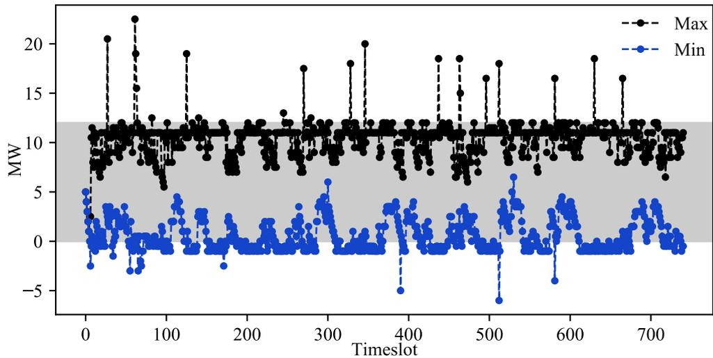
Fig. 3.10 Maximum charge and minimum discharge of the pumped storage by the DDDQN. The shaded area is the safe operational region.
