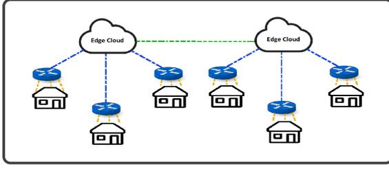
Figure 2: Communications are between IoT to gateways, gateways to edge-clouds and between edge-clouds.
