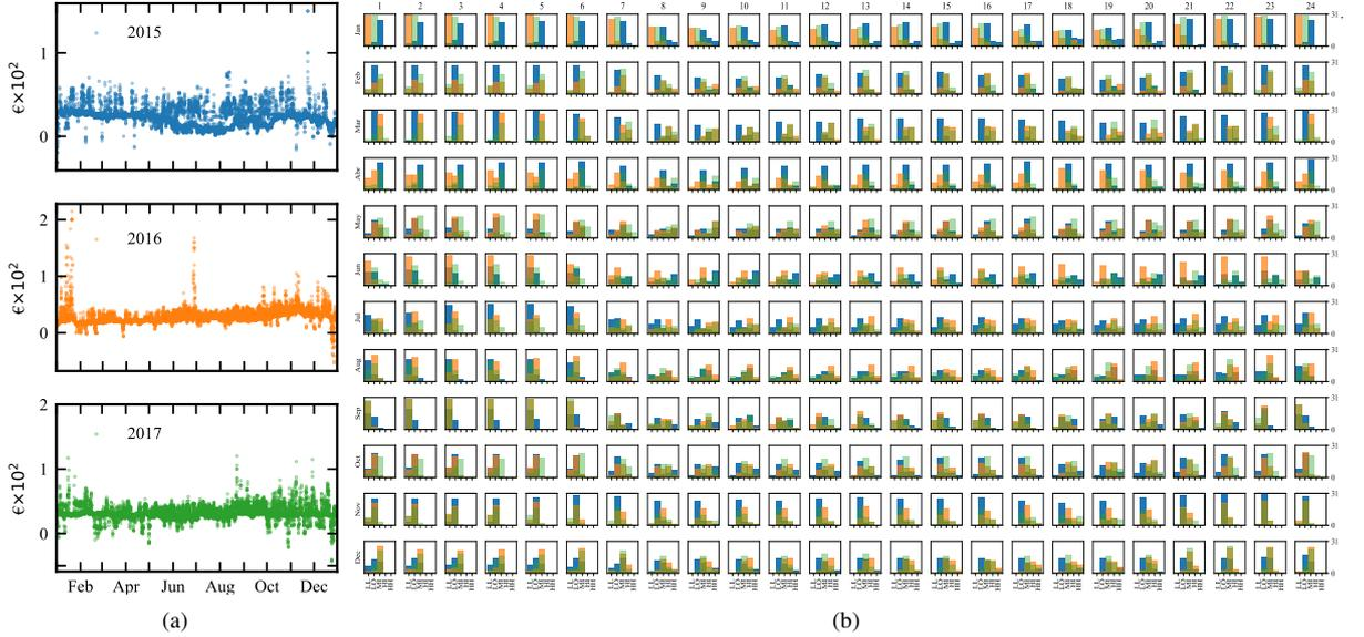
Figure 2: DK2 hourly electricity spot prices from 2015 to 2017. Fig. (a) shows the raw values. Fig (b) shows the histograms of the K-means clusters. 5 clusters are used: Low-low (LL), Low (LO), Mid (MI), High (HI) and High-high (HH).
