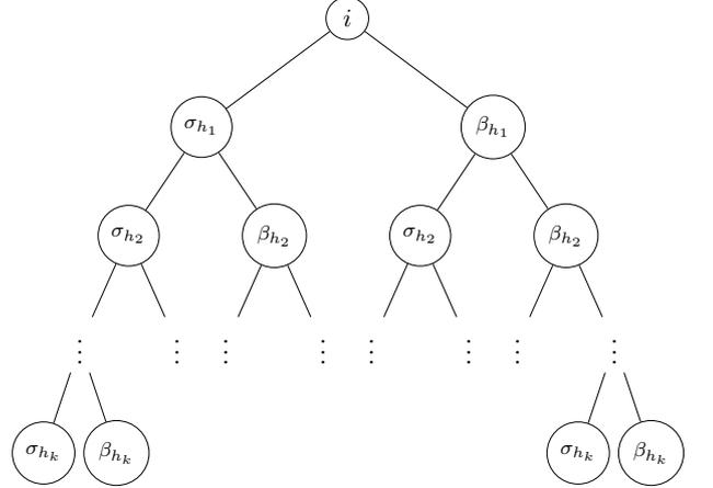
Figure 1: The joint probability of players' pure strategies is recursively computed using a binary tree structure. The inner nodes represent the pure strategies of the players in set  $-i$ , i.e., all other players in  $\mathcal{N}$  but  $i$ .
