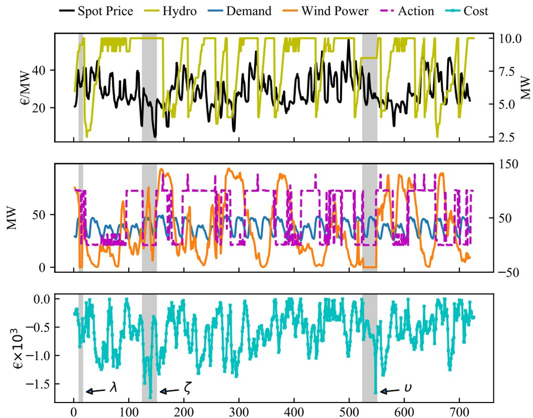
Fig. 3.13 Management of the HWPP with power outages for July 2017.  $\upsilon$  and  $\zeta$  are the time periods with wind or hydro outage respectively. In  $\lambda$  both plants are out of service. The three plots share the x-axis scale.
