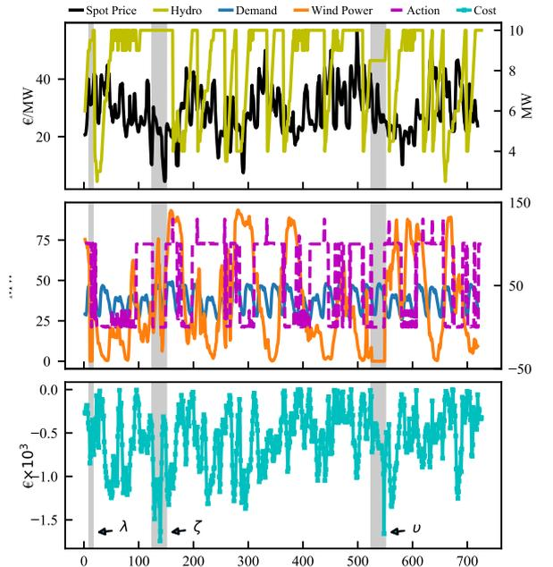
Figure 9<sup>a</sup>: Management of the HWPP with power outages for July 2017.  $\nu$  and  $\zeta$  are the time periods with wind or hydro outage respectively. In  $\lambda$  both plants are out of service.
