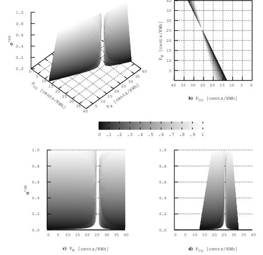
Figure 2. Long-term contracting policy  $\sigma^{*HR}$  for different conventional and wind energy prices with given parameters:  $P_{SM} = 26$  cents/KWh,  $D = 30$  MW and  $\mathbb{E}[w] = 15$  MW.
