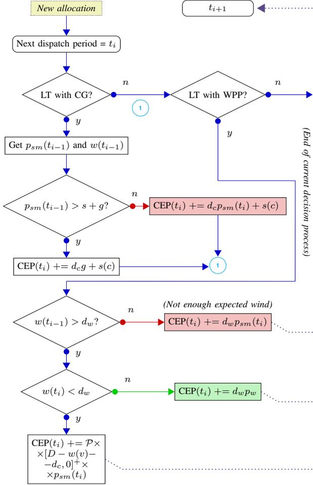
Fig. 3. Flowchart diagram of the LSE procurement decision support algorithm. The drift and diffusion coefficients. This is achieved without sacrificing order of convergence. On the other hand, the drawback is the required multi-step calculations. Nevertheless, given (10) and (11) a derivative free method is preferred.
