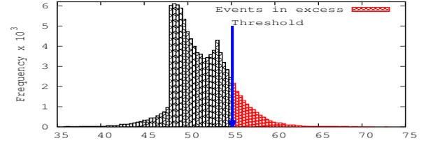
Fig. 4. A process dependent on a random variable can be evaluated by the probability that the random variable surpasses a threshold.
