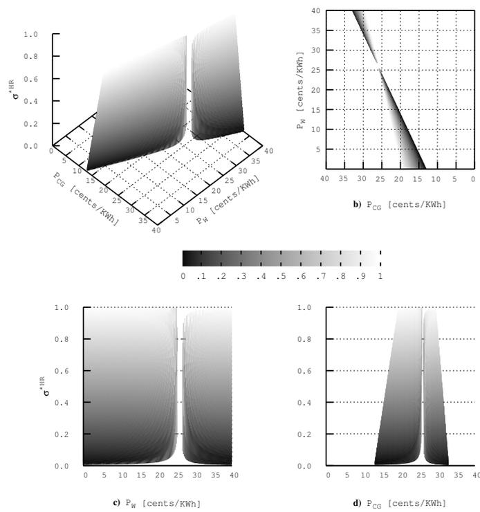
Fig. 3.1 Long-term contracting policy  $\sigma_i^{*HR}$  for different conventional and wind energy prices with given parameters:  $P_{SM} = 26$  cents/KWh,  $D = 30$  MW and  $\mathbb{E}[w] = 15$  MW.
