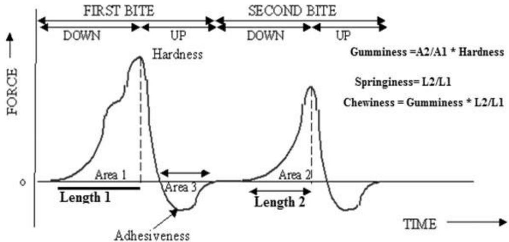
Figure 1.3: A typical texture profile analysis (two-bite force) curve (Banjare, Manikant, Geol, & Uprit, 2015).
