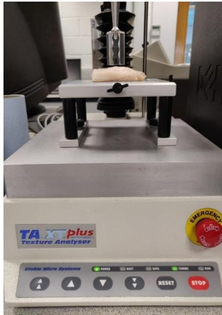
Figure 2.5: Textural analysis of pollack fillets using a TA.XT2i Texture analyser.
