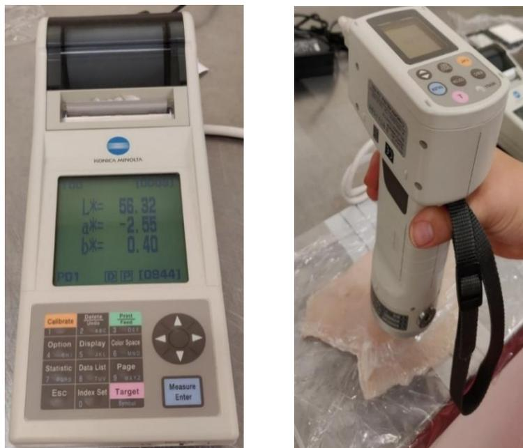
Figure 2.4: Colour analysis of megrim fillets using a Chroma Meter CR-400.
