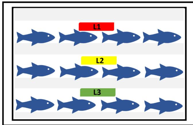
Figure 2.2: Colour coded temperature logger distribution within a polyethylene box containing fish and ice.
