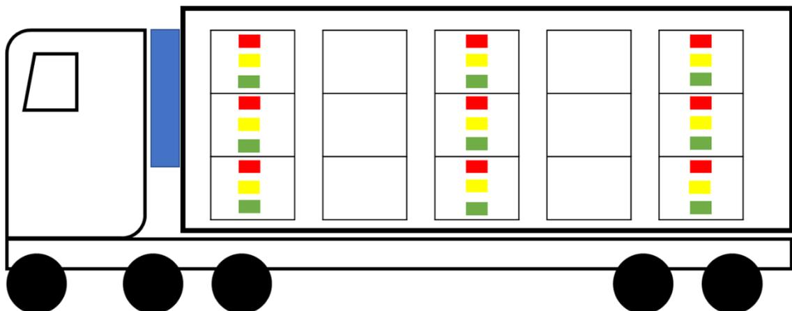
Figure 2.3: Experimental side view setup of the temperature loggers in a distribution truck.
