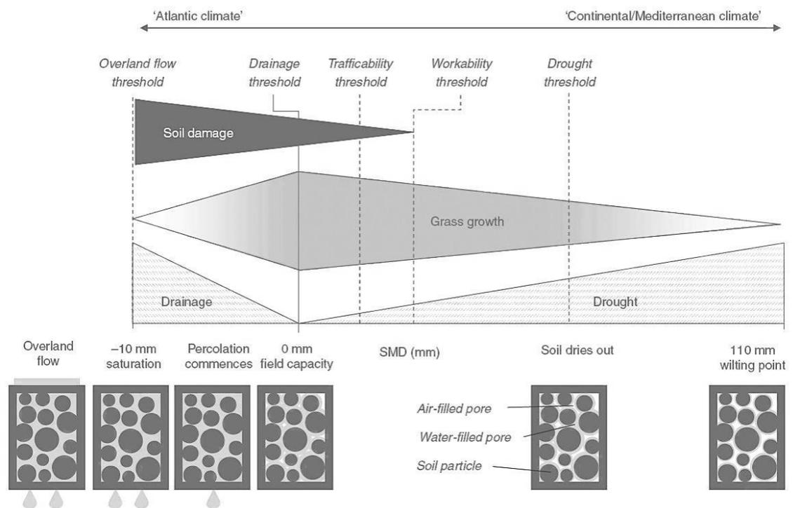
Figure 2.6: Effect of soil moisture deficit on grass growth and soil damage potential (Schulte et al., 2012)
