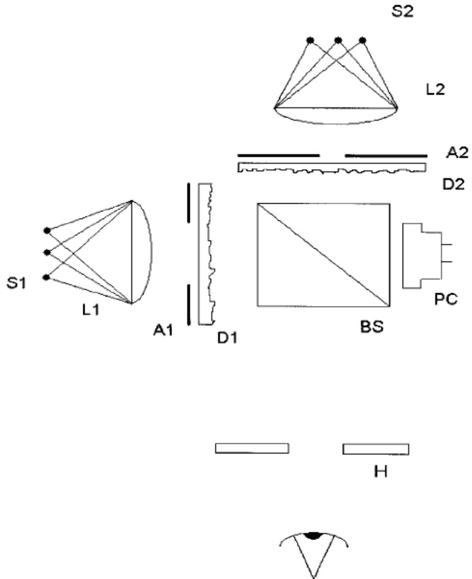
**Figure 2.18** A schematic of the optical system used to measure MPOD in free view in the Macular Densitometer<sup>TM</sup>. A1 and A2: apertures 1 and 2; BS: beam splitter; L1 and L2: planoconvex achromatic lenses; PC: photocell; H: hot mirror used to reduce heat transmission; S1 and S2: light sources; D1 and D2: optical diffusers. [From Wooten *et al.* 1999]<sup>31</sup>
