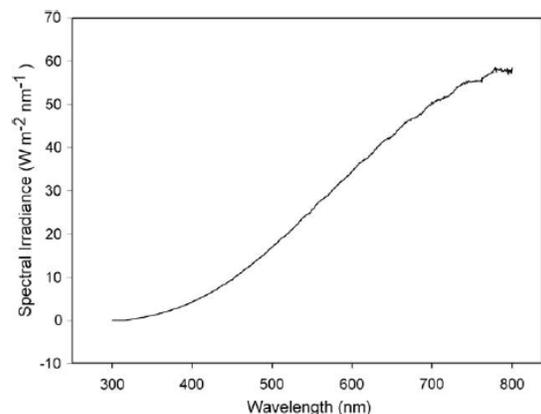
Fig. 1. Spectral Irradiance at 1 m fixation distance from Arri 300 photostress lamp.
