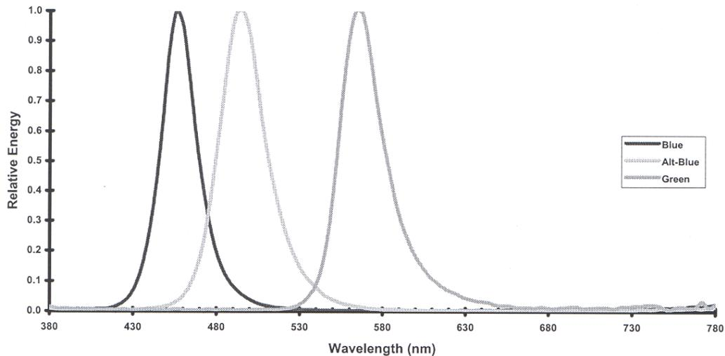
**Figure 2.19** The relative spectral energy curve of the LEDs that were used in the Macular Densitometer<sup>TM</sup>.
