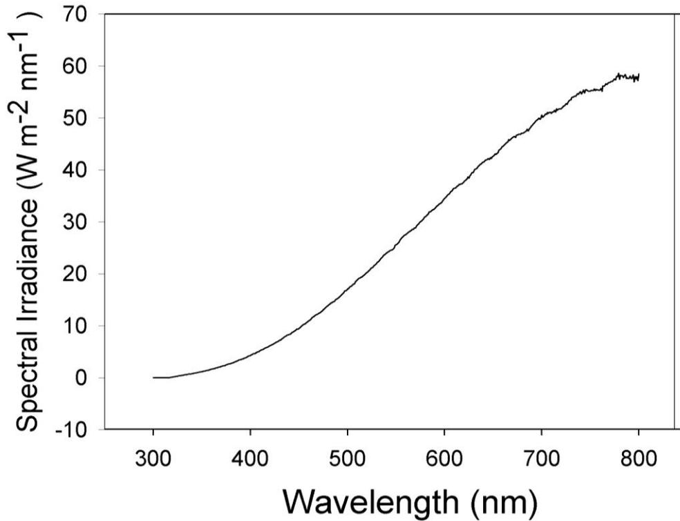
**Figure 2.11** Spectral Irradiance at 1 metre fixation distance from Arri 300 photostress lamp.
