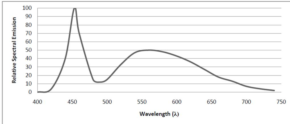
**Figure 2.4** Spectral irradiance profile of the Functional Vision Analyzer™ LEDs, measured with a Bentham DMc 150 Double Monochromator Scanning Spectroradiometer (measured at the plane of the subject’s pupil).
