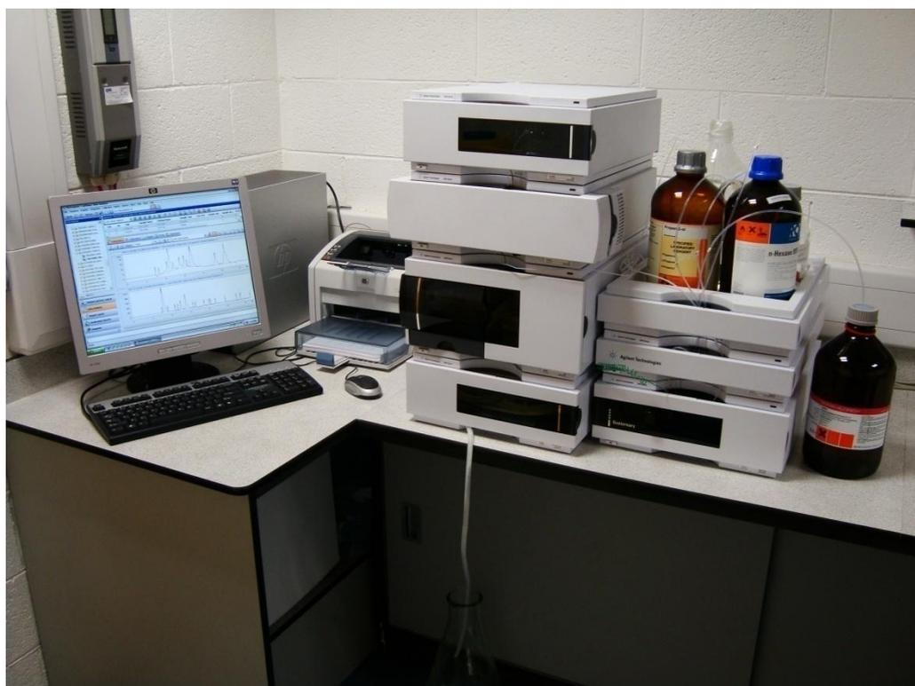
**Figure 2.13** The Agilent 1200 series HPLC system used for analysing L and Z.
