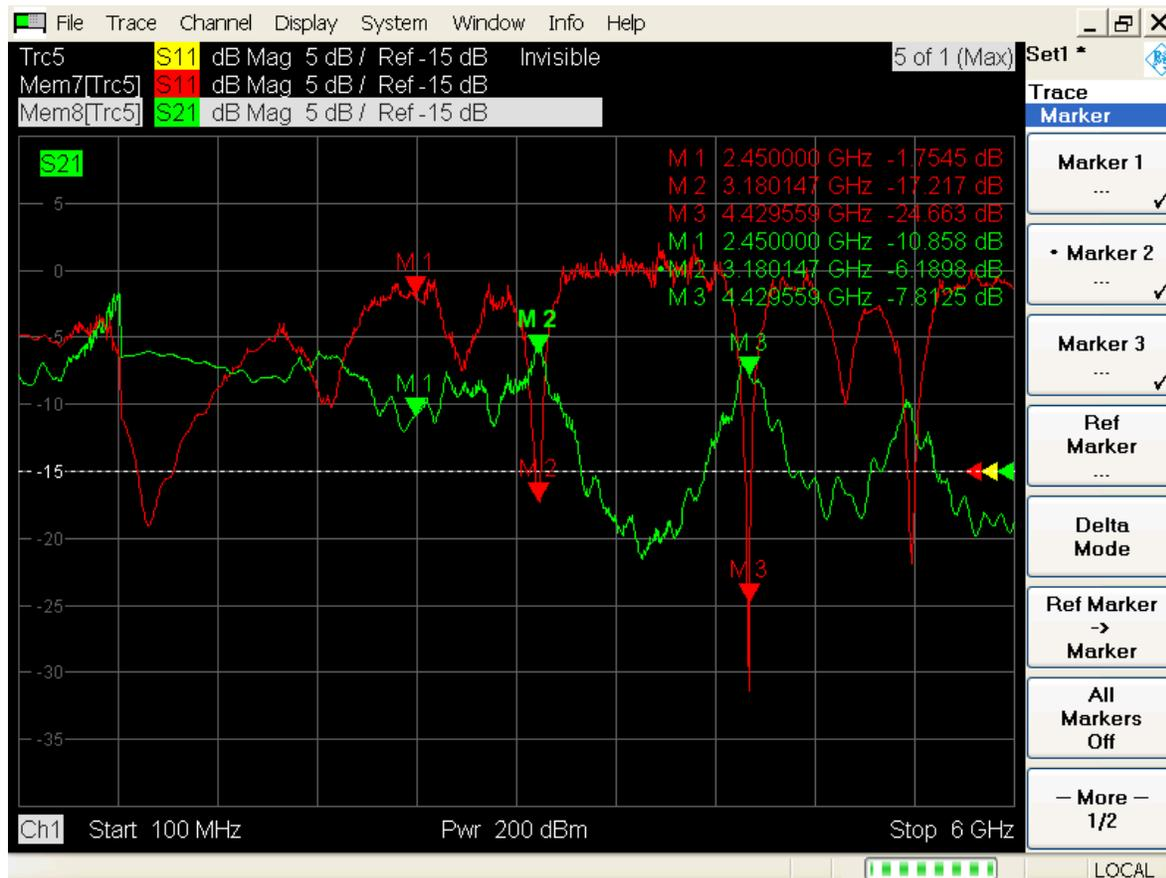
Figure 4.12: Wilkinson Power Divider VNA Measurements
