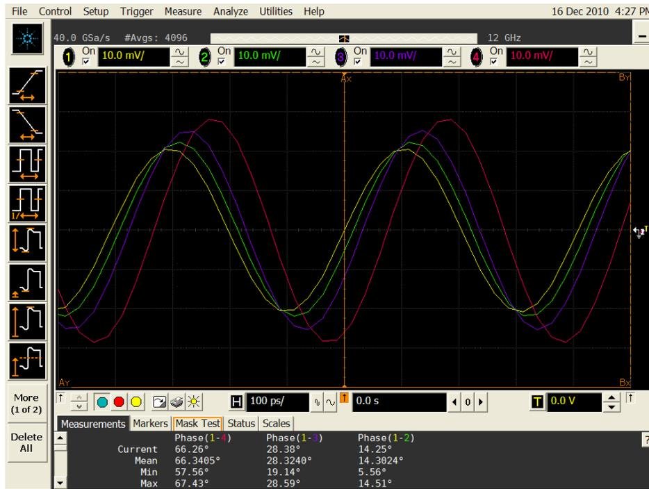
Figure 5.1: Practical Quadrature Modulator Outputs
