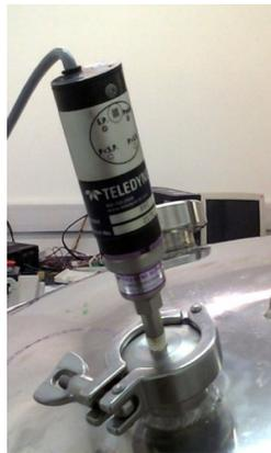
Fig. 193 Teledyne Hastings active vacuum control gauge.
