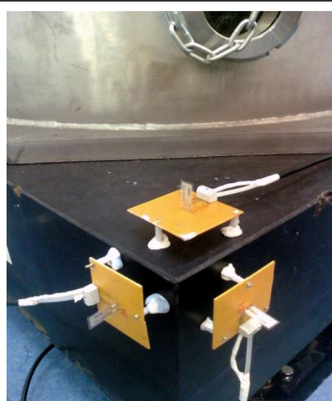
Fig. 195 MSIUSA™ piezo film vibration sensors orientated orthogonal to each other on the granite block.
