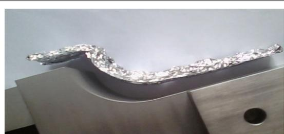
Fig. 189 Thermal shield made from crumpled kitchen foil.
