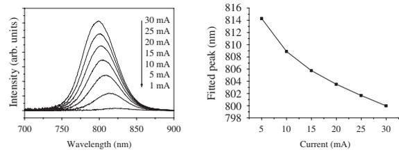
Fig. 1. (a) Amplified Spontaneous Emission (ASE). (b) Peak emission (ASE) as a function of current.
