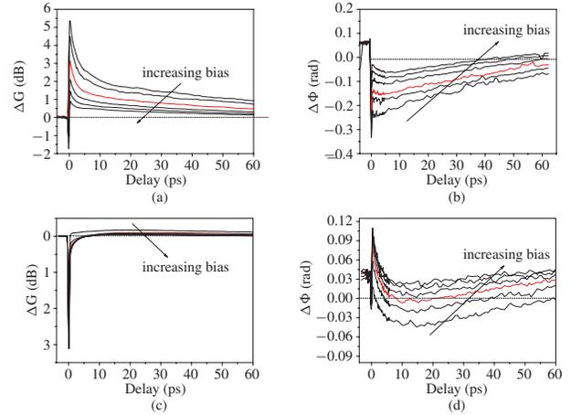
Fig. 4. Detuned pump-probe measurements at 775 nm for (a) gain and (b) phase and at 825 nm for (c) gain and (d) phase. The average pump power was 1 mW, the case corresponding to transparency at 800 nm is shown in red and measurements were taken up to twice this level (from 2 mA to 30 mA).
