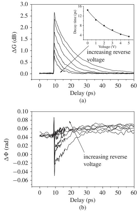
Fig. 6. Gain (a) and phase (b) dynamics in reverse bias mode 800 nm. The reverse voltage range was 0–5 V and pump power was 1 mW. The inset shows the dependence of the single exponential recovery time on voltage.
