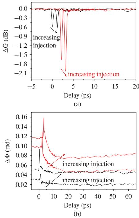
Fig. 5. Pump probe measurements at 850 nm at average pump powers of 1 mW (black) and 3 mW (red) for injection levels of 2 mA and 30 mA. (a) Gain data (offset horizontally for clarity) (b) Phase data (offset vertically for clarity).
