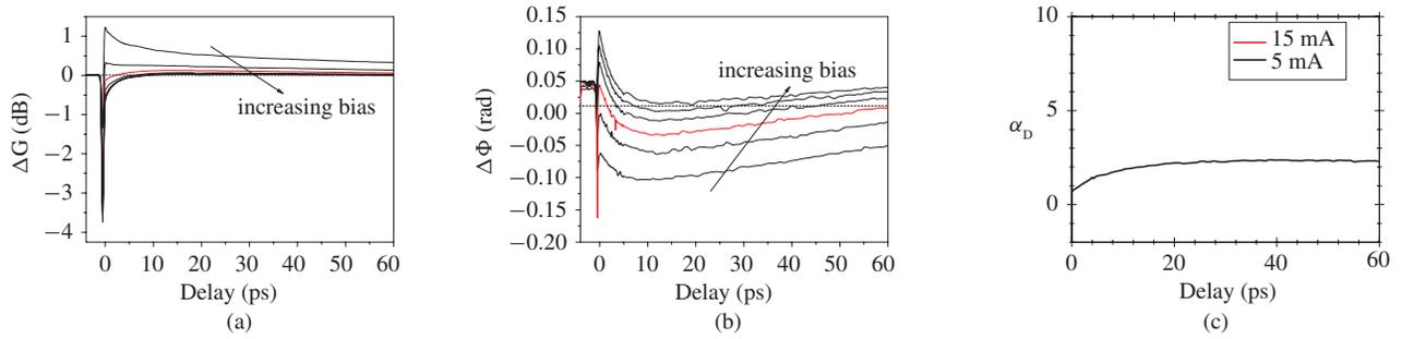
Fig. 3. Gain (a), phase (b) and alpha-factor (c) dynamics following the injection of pump pulse of average power 1 mW. The transparency case is shown in red and measurements were taken up to twice transparency (from 2 mA to 30 mA).
