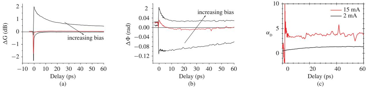
Fig. 2. Gain (a), phase (b) and alpha-factor (c) dynamics following the injection of pump pulse of average power 0.5 mW. The transparency case is shown in red and measurements were also taken at 2 mA and 30 mA.
