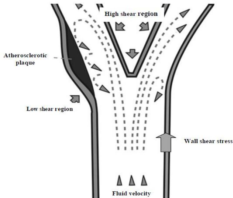
*Figure 1.8: Wall shear stress with boundary layer separation*
