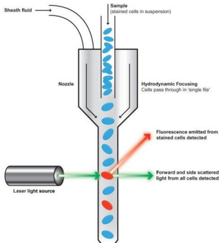
Figure 1.18: The principles of flow cytometry
