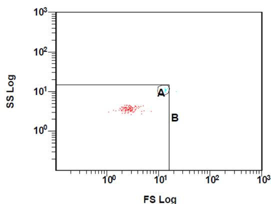
Figure 2.3: FS Log/SS Log plot used for size calibration and gating. A is the population of  $0.9 \mu\text{m}$  beads and B is the gate that represents all events  $<1.0 \mu\text{m}$ . FS; forward scatter, SS; side scatter
