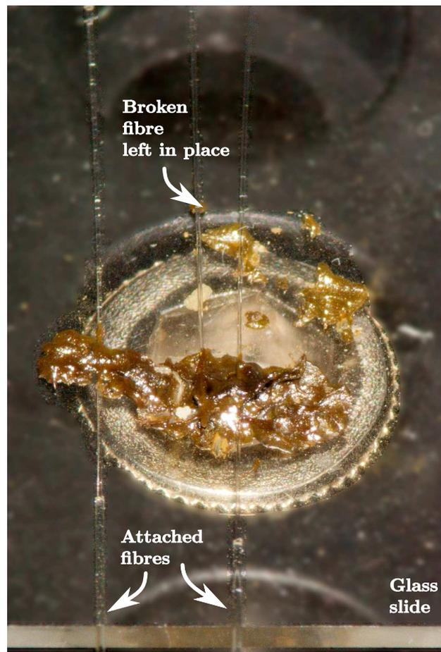
**Figure 4.17:** Close up image of soldered fibres.
