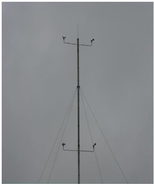
Figure 2 Wind sensors located at 6m and 10m
