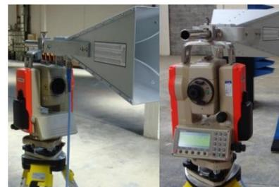
Figure 2 Modified Total Station Antenna Mount
