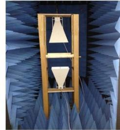
Fig. 9: Candidate vertical measurement system
