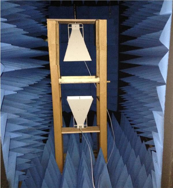
Figure 5-38 Vertical measurement system, photo shoot in WIT anechoic chamber
