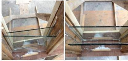
Fig. 4: Container wall's misalignment
