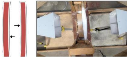
Fig. 6: Lens effect caused by insufficient container rigidity
