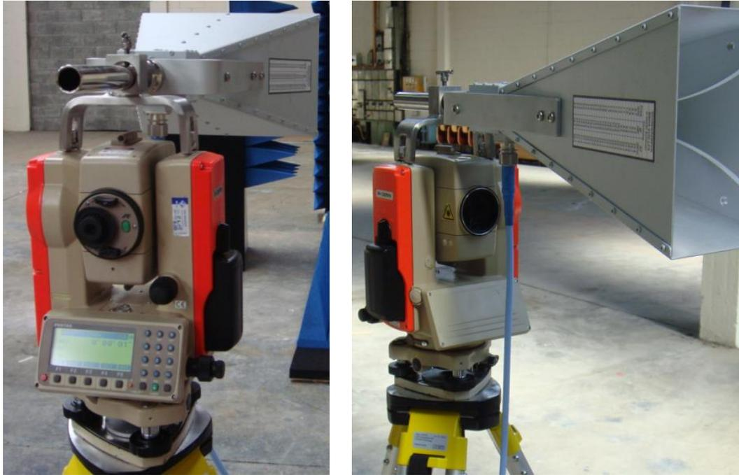
Figure 3-3 Modified Pentax Total Station for antenna mounting
