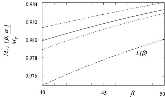
Fig. 3. The reduced parallel magnetisation  $M_{\parallel}(\alpha, \beta)/M_s$  for aligned particles  $\alpha = 5$ . The solid is from the single integral forms. The dashed curve is  $L(\beta)$ . The dotted and the dot-dashed curves are Eqs. (32) and (34), respectively.
