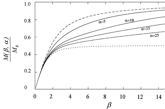
Fig. 2. The reduced magnetisation  $M(\alpha, \beta)/M_s$  as a function of  $\beta = HM_s V/kT$  for a system with random texture. The dashed and dotted curves are  $L(\beta)$  and Eq. (40), respectively. The solid lines are calculated numerically using the single integral forms Eqs. (7) and (8) with Eqs. (1) and (3), for  $\alpha = 5, 10, 15$  and  $25$ .
