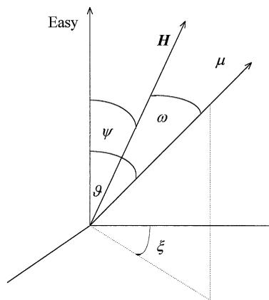
Fig. 1. The coordinate system used, with particle easy axis, field  $H$  and moment  $\mu$ .
