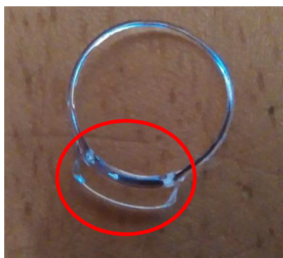
Figure 2.7: Polymerised excess monomer removed from the contact lens polypropylene mould post polymerisation.
