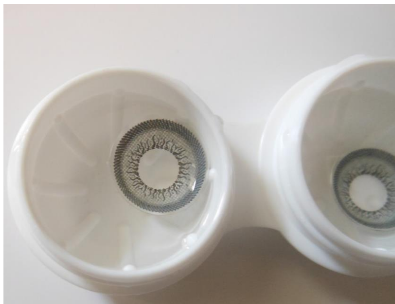
Figure 1.10 Image of contact lens being drug loaded via soaking.
