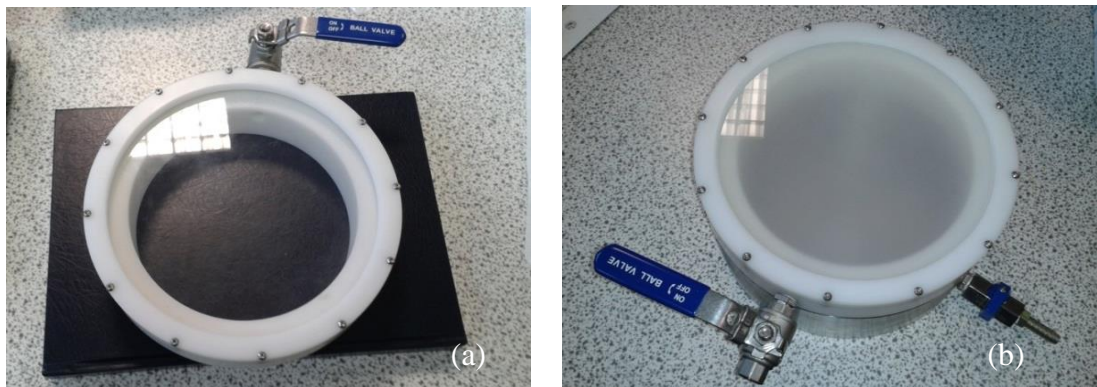
Figure 2.3: Polycarbonate UV transmissible window (a) and separate UV diffuser (b).
