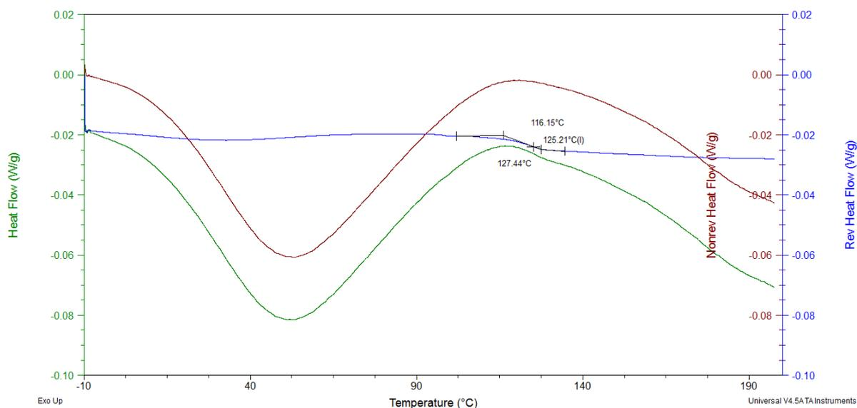
Figure 6.18 MDSC thermogram of 5% TPAAm with the addition of CPM
