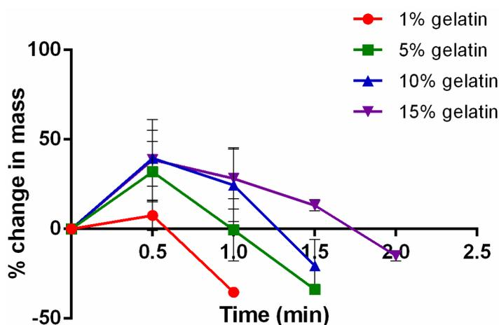
Figure 5.6 Swelling studies of unmodified PAAm with the addition of varying levels of gelatin
