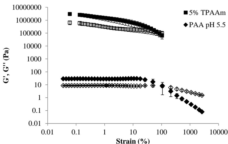
**Figure 6.4** Strain sweep of 5% TPAAm and thiolated PAA pH 5.5, displaying both G' (closed symbols) and G'' (open symbols) values (n=2)
