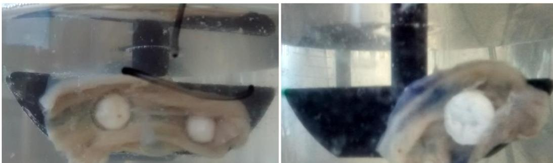
**Figure 5.10 Mucoadhesive testing of thiolated PAA samples, pH 6 and pH 5.5 (left) and 5% TPAAm sample (right) after 10 min**
