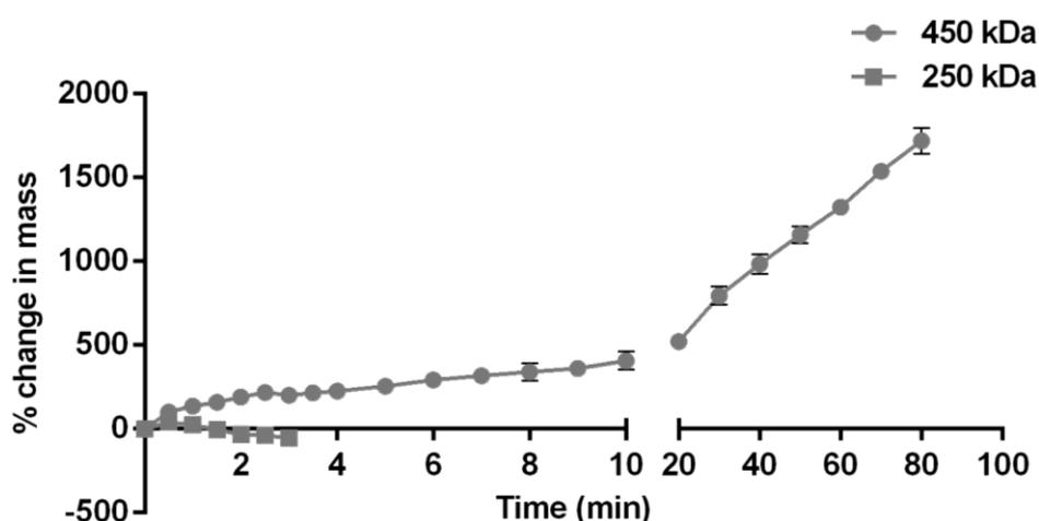
Figure 2.7 Swelling tests on thiolated PAA of two molecular weights, 250 kDa and 450 kDa (n=2). Both samples had comparable thiol content measuring  $437.5 \pm 3.1 \mu\text{mol/g}$  and  $472.4 \pm 28.2 \mu\text{mol/g}$ , respectively.
