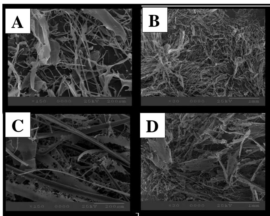
Figure 2.17 SEM images of thiolated PAA (A and B) and thiolated PAA-CPM conjugate (C and D) at magnifications of 150 on the left and 30 on the right
