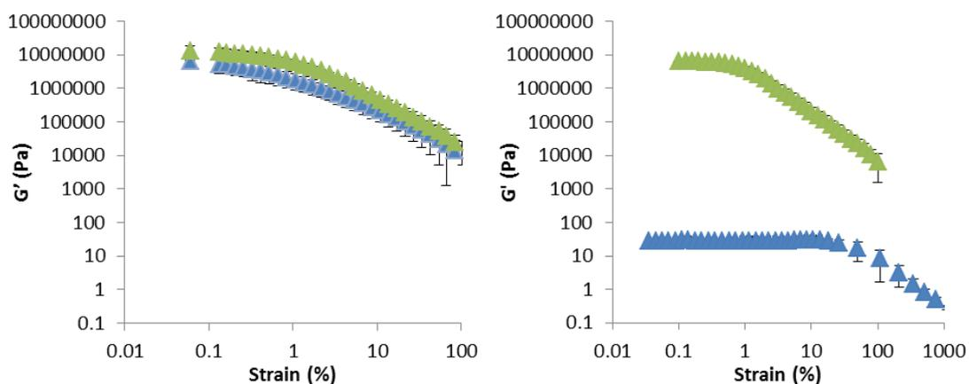
**Figure 6.6**  $G'$  values of polymer samples with (green) and without (blue) mucin addition. 2.5% TPAAm is on the left and PAA pH 5.5 is on the right ( $n=2$ )
