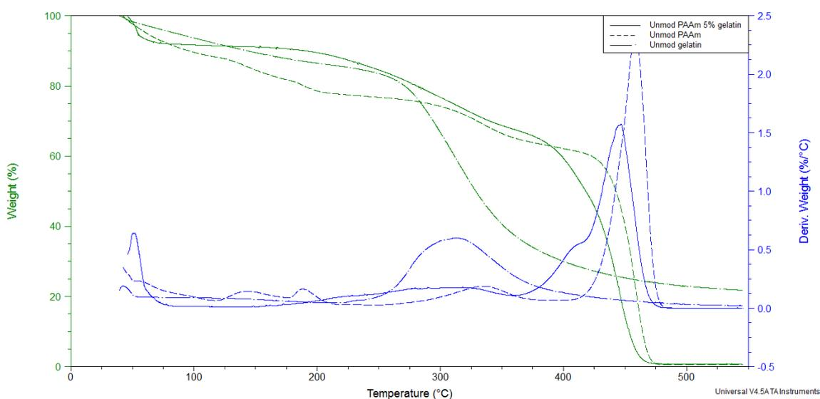
**Figure 6.12 TGA of unmodified PAAm, unmodified gelatin and PAAm/5% gelatin**
