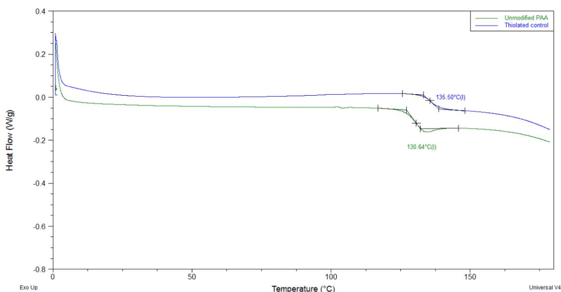
**Figure 2.20 DSC curve showing the 2nd heat cycle of unmodified and thiolated control PAA.  $T_g$  values are labelled.**
