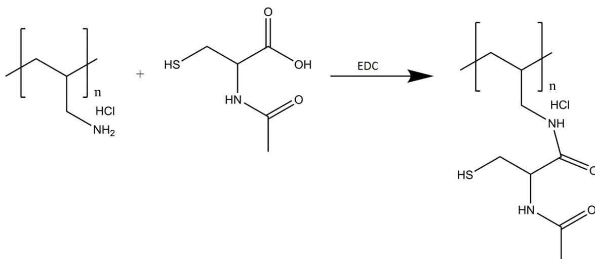
**Figure 5.2** Thiolation reaction of PAH and N-acetyl cysteine and the crosslinker, EDC (Vigl *et al.*, 2009)
