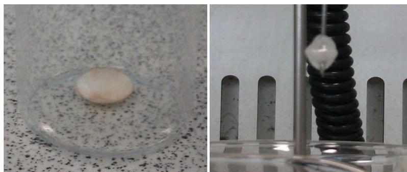
**Figure 4.17** Images of gelatin sample as a dry tablet, approximately 1 cm in diameter (left) and swollen during swelling tests after approximately 10 min in buffer (right).
