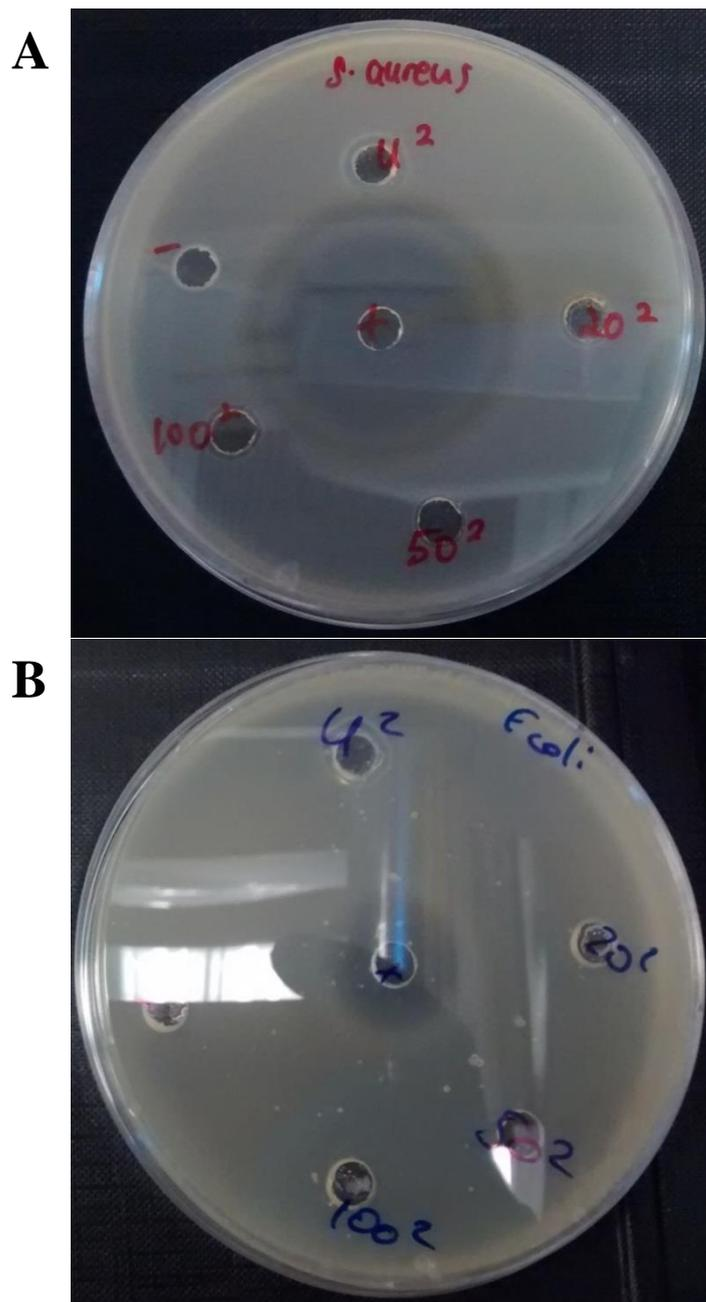
**Figure 6.20** Antimicrobial testing against *S. aureus* (A) and *E. coli* (B) using unmodified and thiolated PAAM samples at a concentration of 2 mg/mL.
