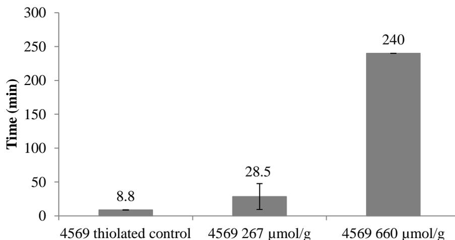
**Figure 4.13 Mucoadhesive testing of gelatin 4569: thiolated control (n=3), with thiol content of 267  $\mu\text{mol/g}$  (n=2) and with thiol content of 660  $\mu\text{mol/g}$  (n=1). Samples were aminated at pH 5**
