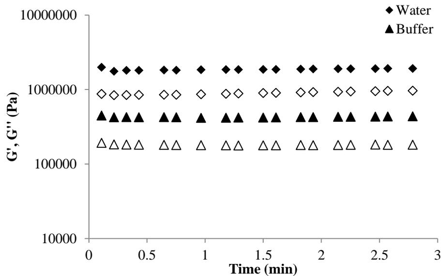
**Figure 6.9** Time sweeps displaying the  $G'$  (closed symbols) and  $G''$  (open symbols) of 1% TPAAM made in water and in buffer over the initial 3 min ( $n=2$ )
