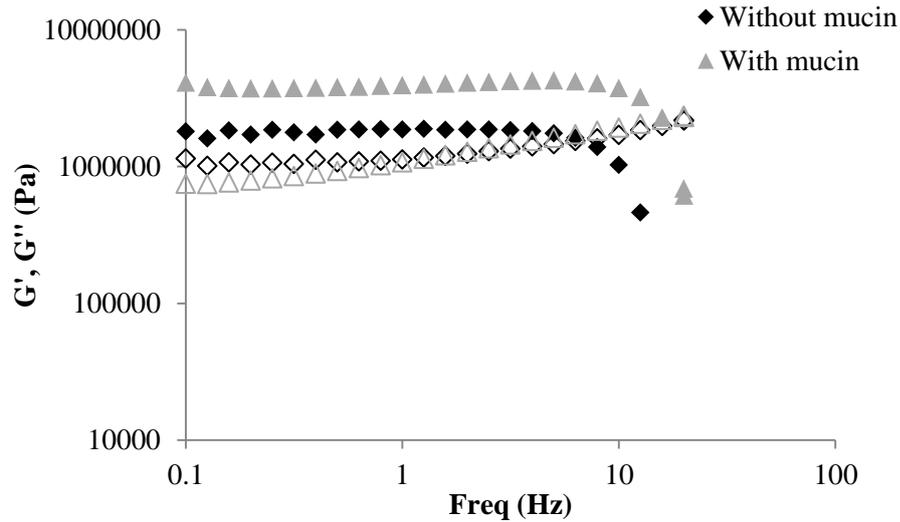
Figure 6.7 Frequency sweep of 2.5% TPAAm with and without mucin displaying G' (closed symbols) and G'' (open symbols) values (n=2)
