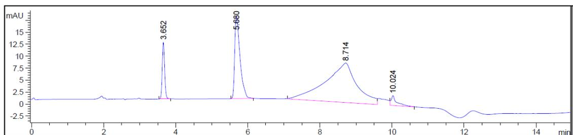
**Figure 6.1** Typical chromatogram the release of CPM from thiolated PAAm, displaying the maleate peak eluting at 3.6 min and the chlorpheniramine peak eluting at 5.6 min.
