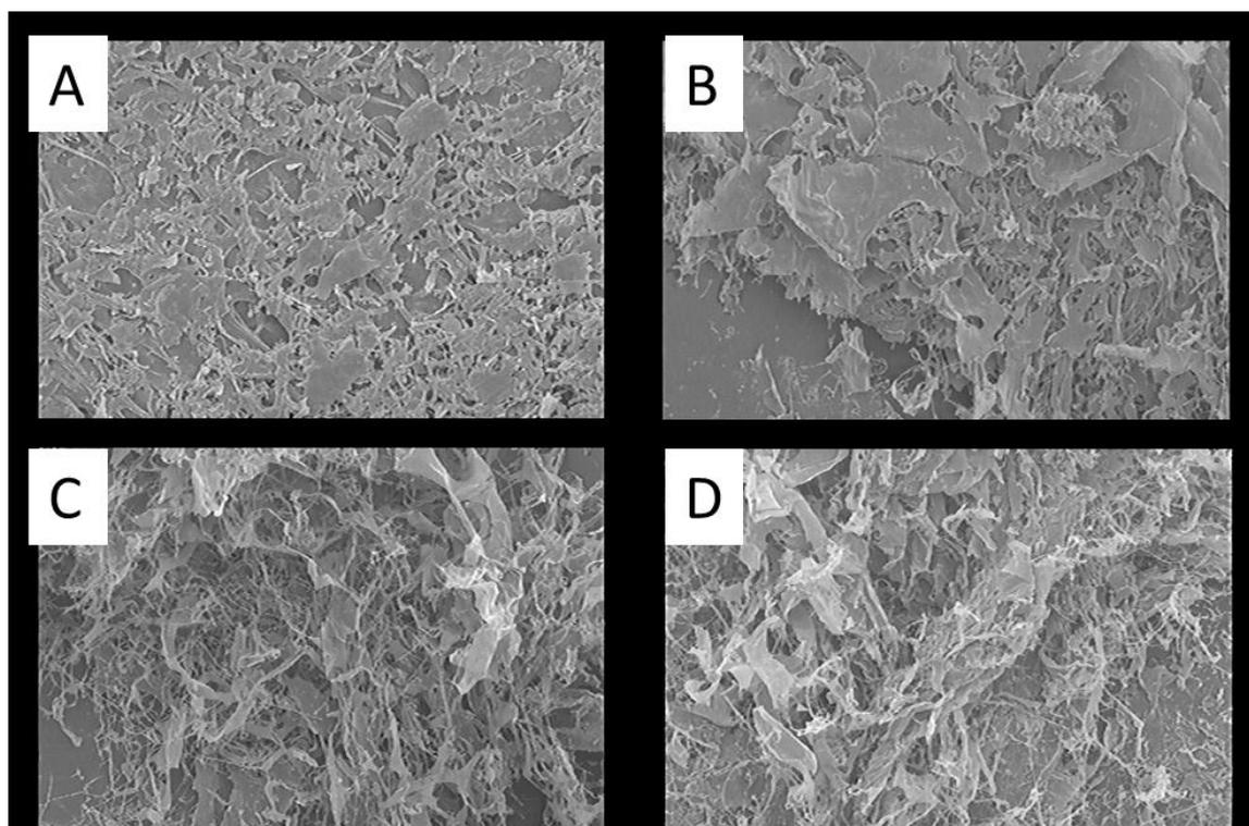
Figure 6.11 SEM imaging of (A) Unmodified/5% gelatin PAAm, (B) 1% TPAAm, (C) 2.5% TPAAm and (D) 5% TPAAm
