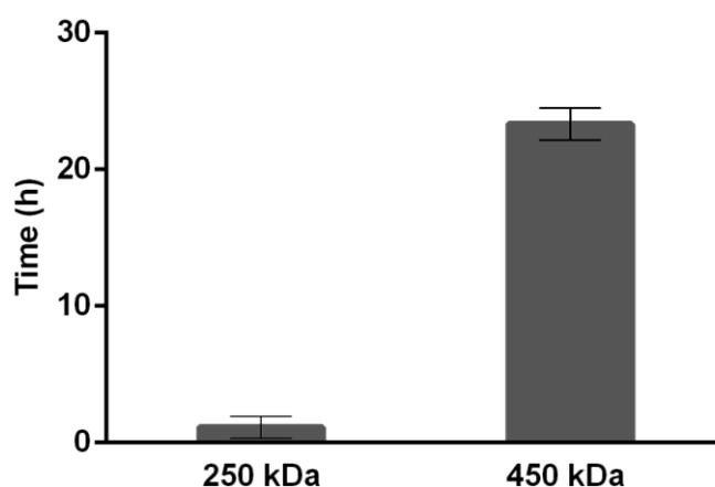
**Figure 2.10** Mucoadhesive testing on thiolated PAA samples of comparable thiol content ( $\sim 450 \mu\text{mol/g}$ ) but differing MW, 250 kDa and 450 kDa (n=3)
