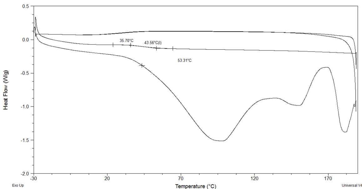
**Figure 6.15 DSC thermogram, displaying the heat-cool-heat-cool cycles of unmodified PAAm**
