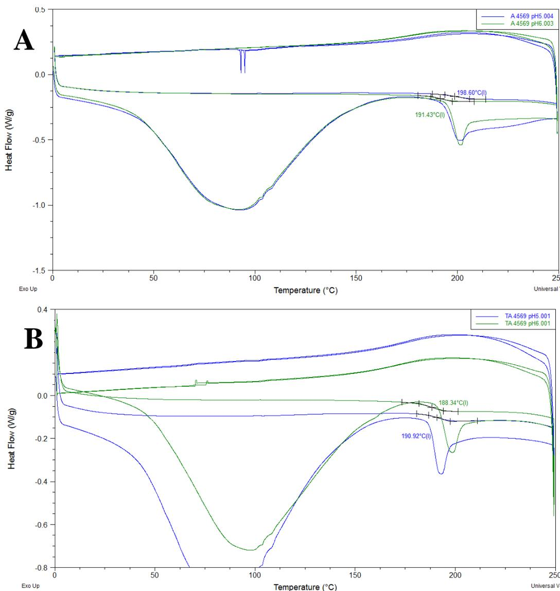
Figure 4.22 DSC curves of gelatin 4569 aminated at pH 5 and pH 6: (A) aminated samples and (B) thiolated samples
