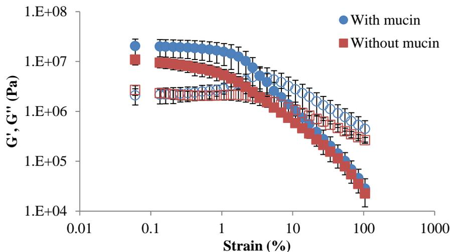
**Figure 6.5**  $G'$  (closed symbols) and  $G''$  (open symbols) values of 1% TPAAm with and without the addition of an 8% mucin solution ( $n=2$ )
