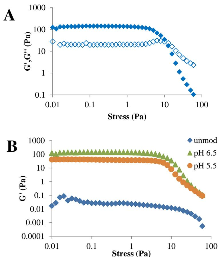
**Figure 2.14 (A) Stress tests of thiolated sample pH 6.5 displaying G' (closed symbols) and G'' (open symbols) values, (B) Stress tests of unmodified PAA and thiolated PAA samples, indicating G' values**
