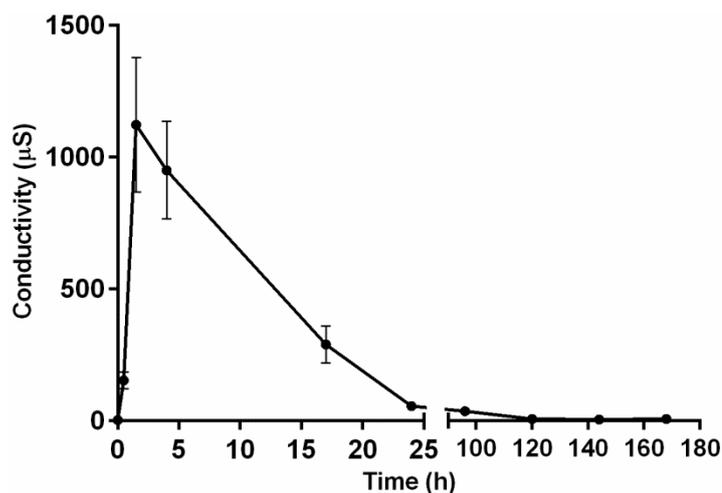
Figure 3.7 Measurement of conductivity during dialysis of aminated gelatin 4567, pH 5 (n=2)
