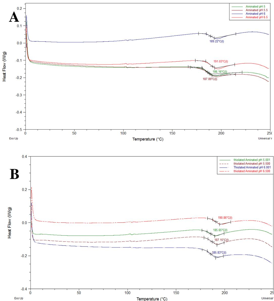
Figure 4.21 DSC curve showing 2nd heating cycle and  $T_g$  of gelatin 4567 (A) aminated at varying pHs and (B) thiolated samples
