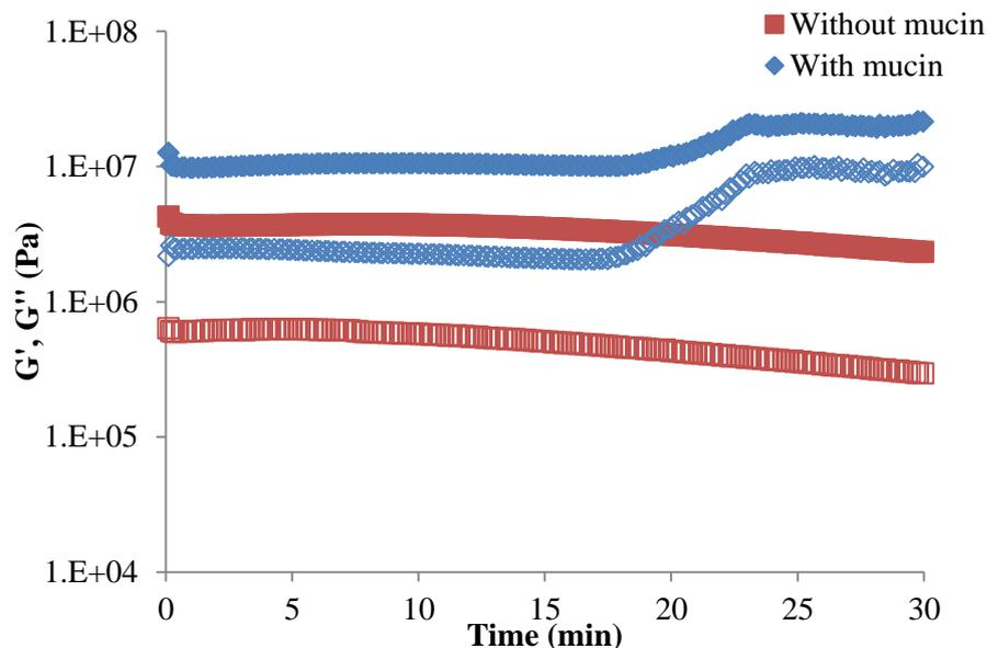
**Figure 6.10** Time sweep of 2.5% TPAAm with and without the addition of mucin, displaying G' (closed symbols) and G'' (open symbols) values (n=2)
