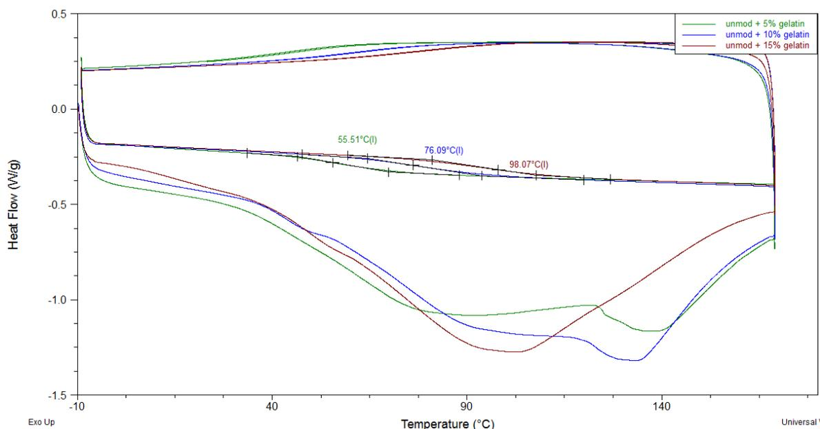
**Figure 6.16 DSC analysis of unmodified PAAm with the addition of gelatin at different ratios**
