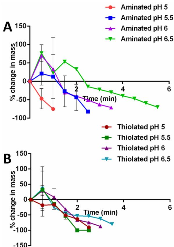
**Figure 4.8 Swelling studies of gelatin 4567 samples aminated at varying pH values, of (A) aminated samples and (B) thiolated samples (n=2)**
