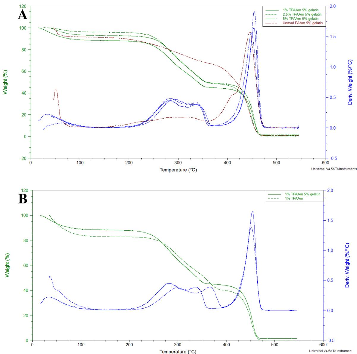
**Figure 6.14 TGA of (A) thiolated and unmodified PAAm with addition of 5% gelatin and (B) 1% TPAAm with and without the addition of gelatin**
