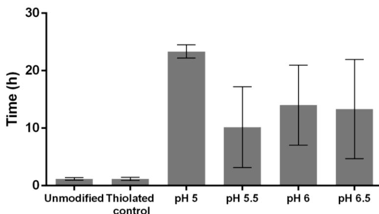
**Figure 2.11 Mucoadhesive testing of unmodified PAA, thiolated controls and thiolated samples of varying thiol content (n=3)**
