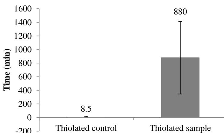
**Figure 4.16 Mucoadhesive testing on thiolated controls (n=2) and thiolated samples (n=3) of gelatin 4569 which had been aminated at pH 6**
