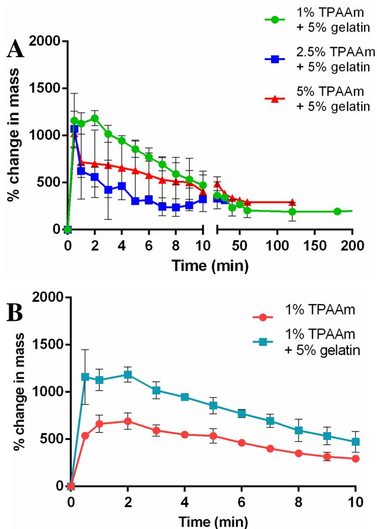
Figure 5.8 Swelling studies of (A) thiolated PAAm samples with the addition of 5% gelatin (n=3) and (B) 1% TPAAm with and without gelatin addition
