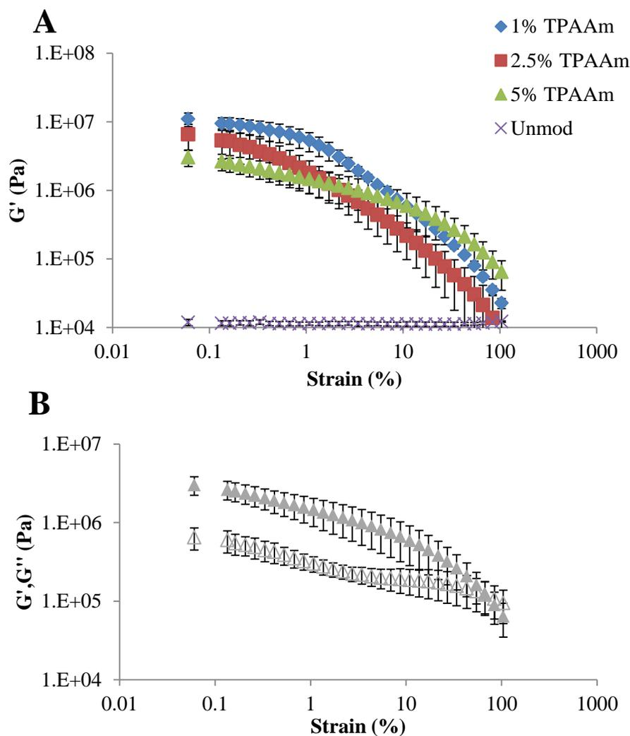
**Figure 6.3** Strain sweep of thiolated PAAM samples displaying (A)  $G'$  values of thiolated PAAM in comparison to unmodified PAAM and (B)  $G'$  (closed) and  $G''$  (open) values of 5% TPAAM ( $n=2$ )
