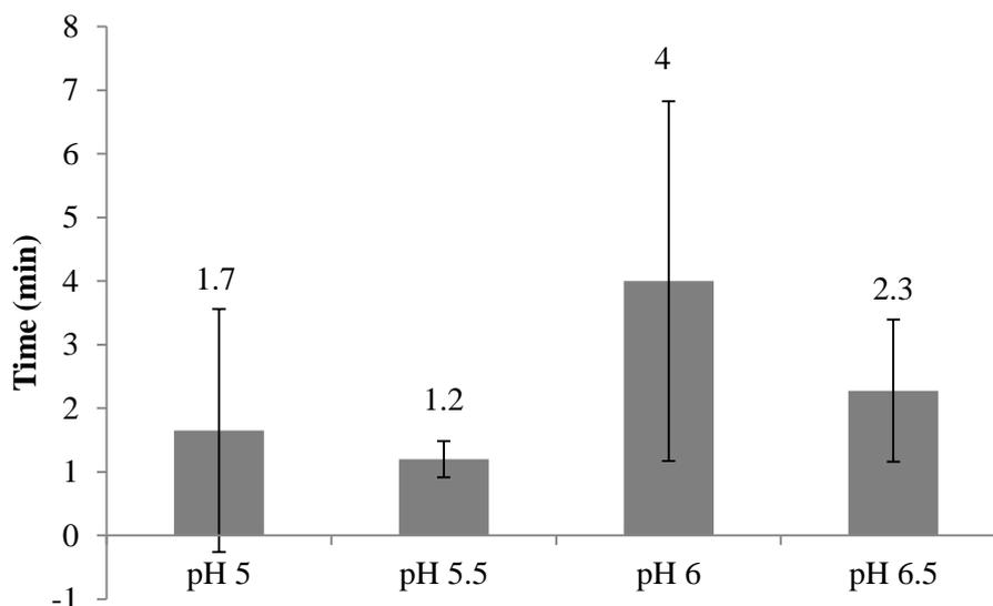
**Figure 4.15 Mucoadhesive testing on thiolated gelatin 4567 samples which were aminated at varying pH values (n=3)**
