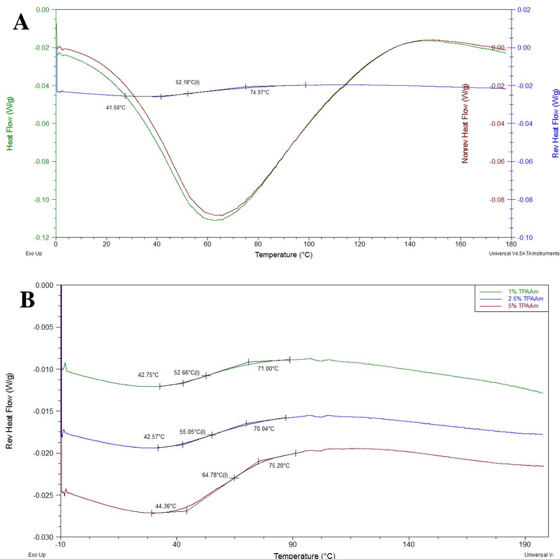
**Figure 6.17 MDSC thermogram of (A) 1% TPAAm displaying the heat flow and reversing and non-reversing heat flows and (B) the reversing heat flow of TPAAm samples, with exothermic peak highlighted**
