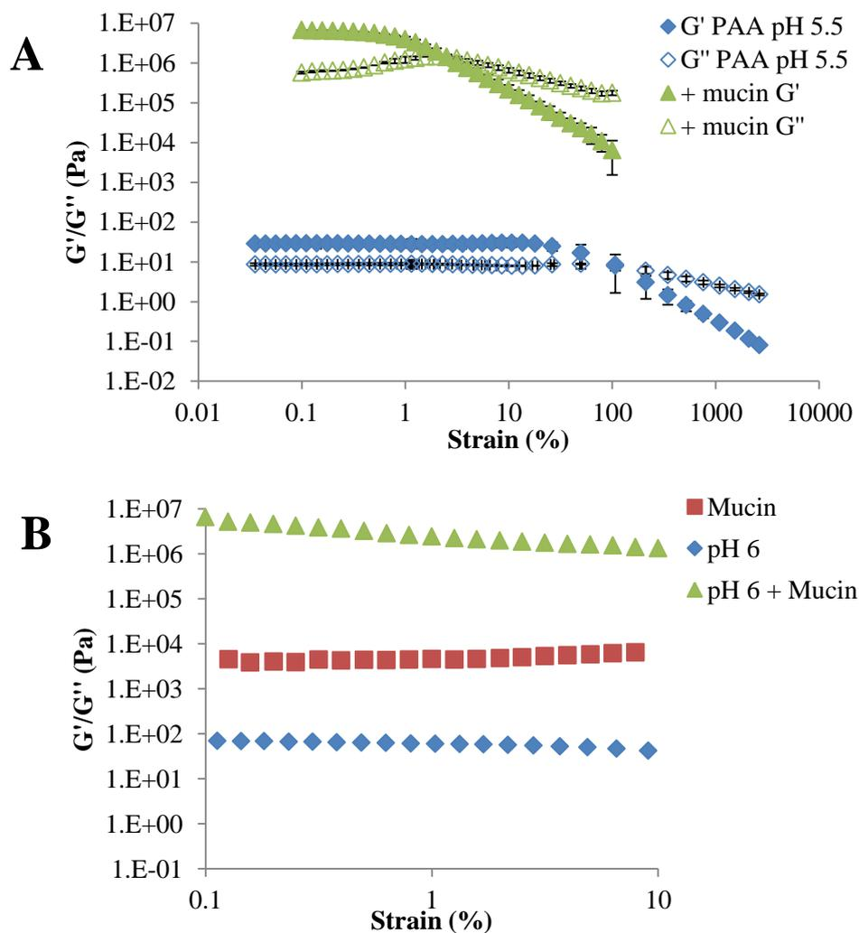
**Figure 2.15** Strain sweeps displaying (A)  $G'$  and  $G''$  values of PAA pH 5.5 with and without the addition of mucin and (B)  $G'$  of PAA pH 6, PAA pH 6 with mucin and mucin alone ( $n=2$ )
