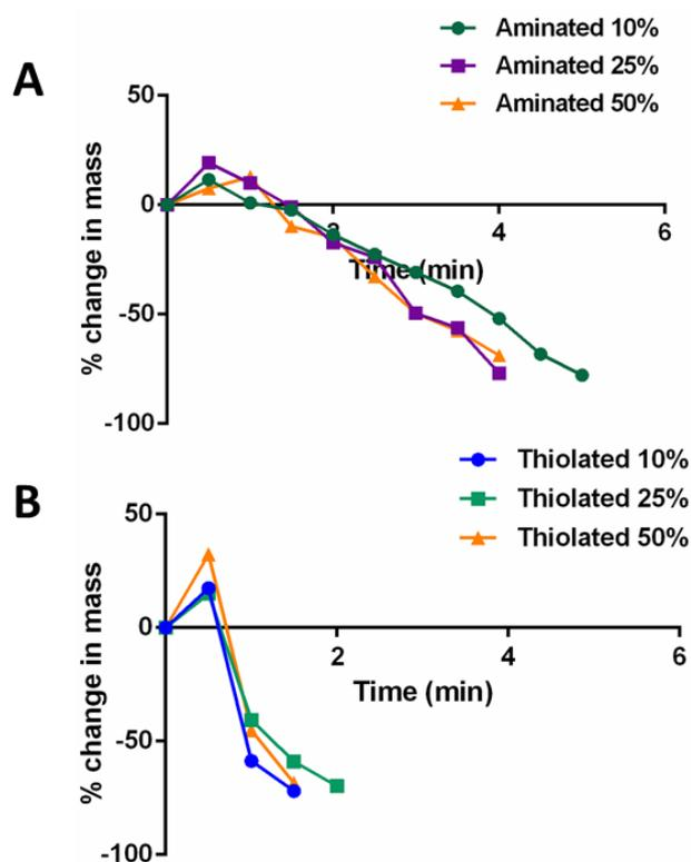
Figure 4.7 Swelling studies on gelatin 4567 samples aminated at varying ethylene diamine concentrations of (A) aminated samples and (B) thiolated samples (n=1)
