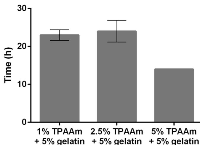
**Figure 5.11** Mucoadhesive testing of TPAAm samples with the addition of 5% gelatin (n=2)
