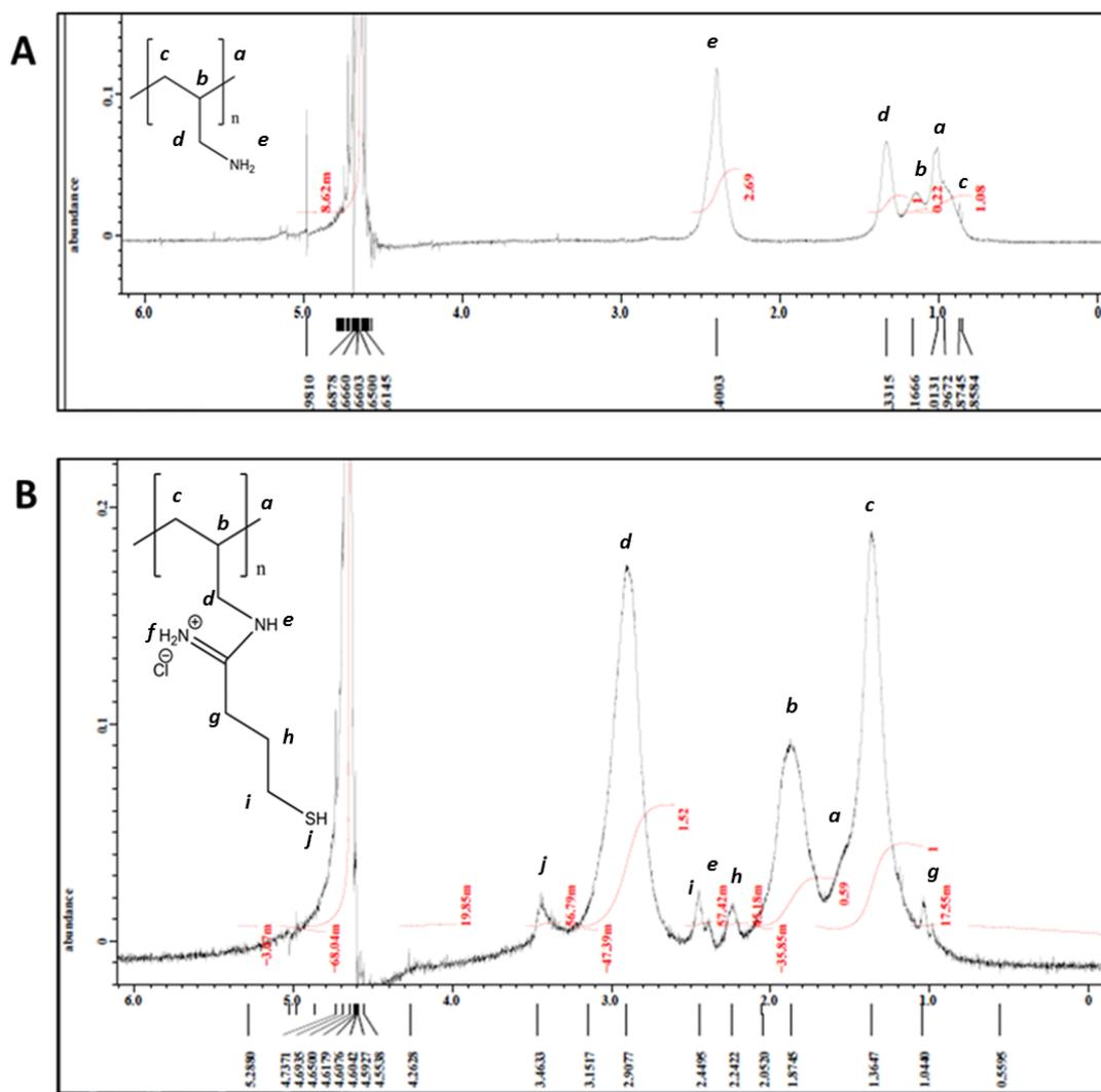
Figure 5.4 NMR spectra of (A) unmodified PAAm and (B) 1% TPAAM
