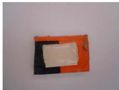
**Figure 2.5** Mousetrap glue patch used in hair tubes
