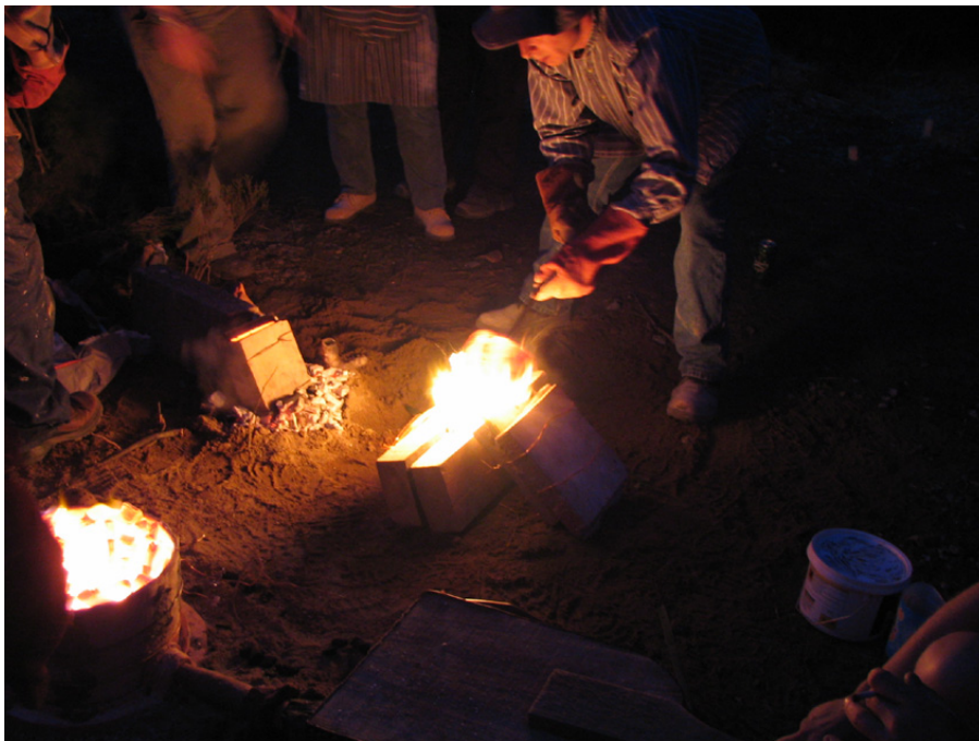
Figure 30: Casting into an experimental wooden mould, using a graphite crucible at An Creagán. Photograph C. Hansen 2006
