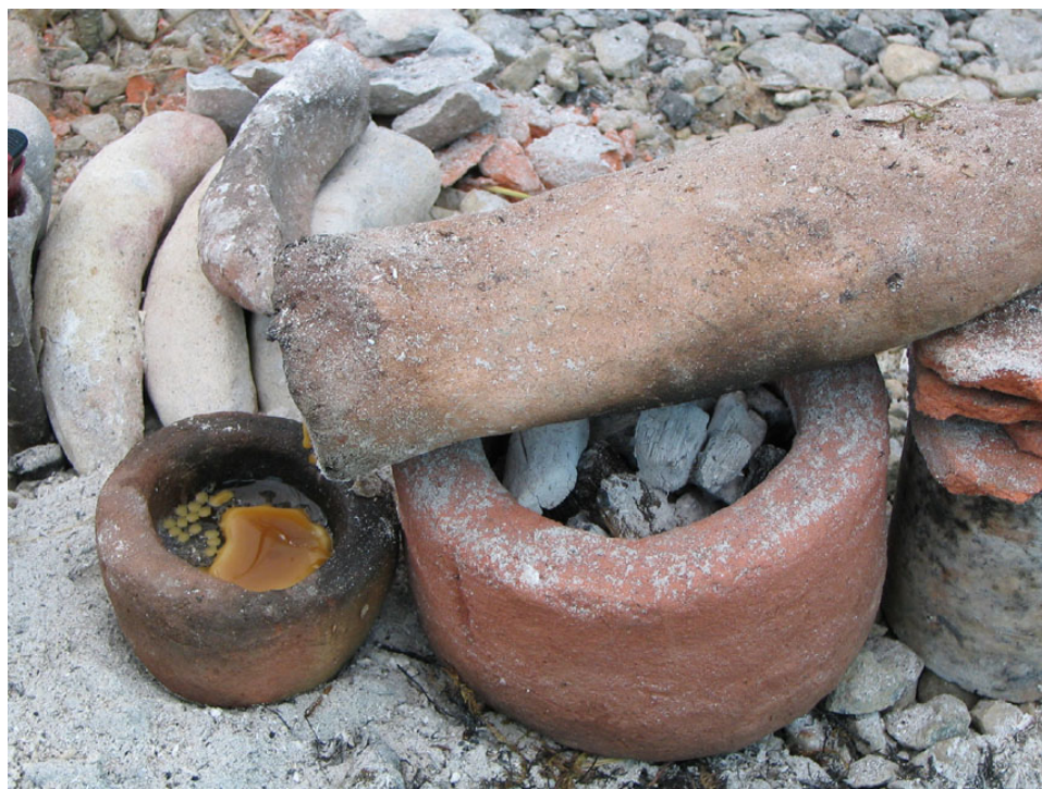
Figure 36: Lost wax mould with charcoal heater by Holger Lönze at An Creagán. Photograph C. Hansen 2006
