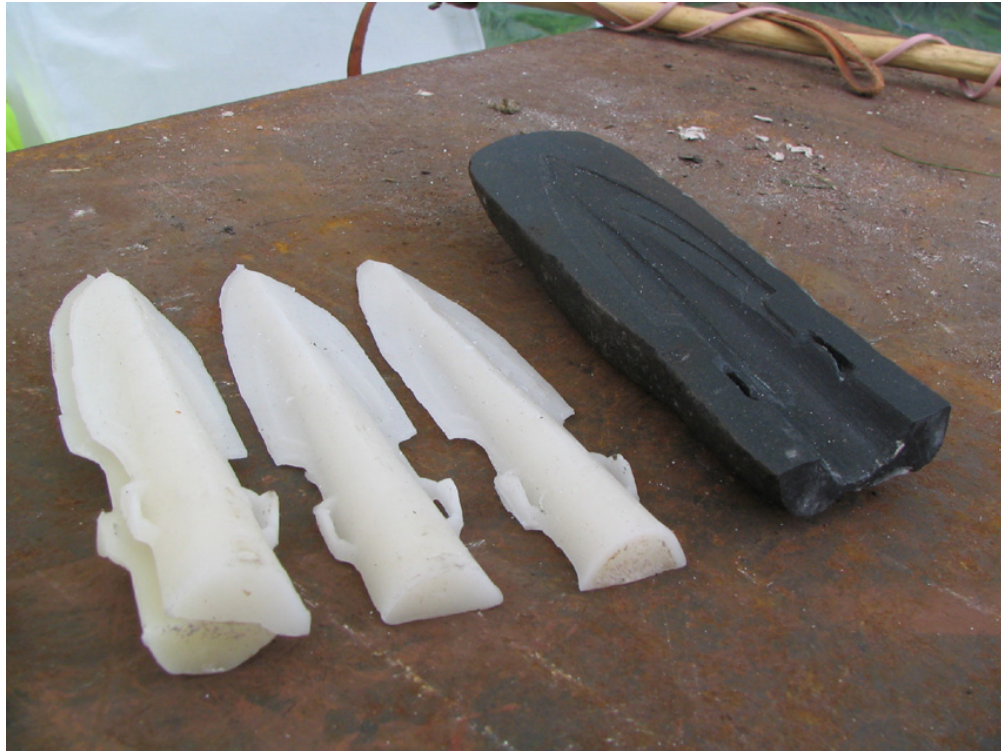
Figure 47: Carved stone mould with wax impressions by Jon Fyffe. Photograph C. Hansen 2006
