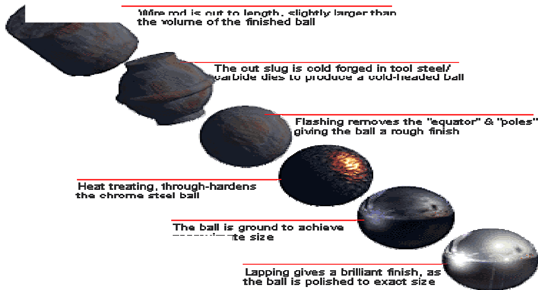
Figure 1-4 The 5 production steps of bearing balls [1]
