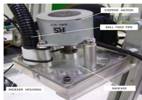
Figure 87 Prototyped Rotary Indexer [24]
