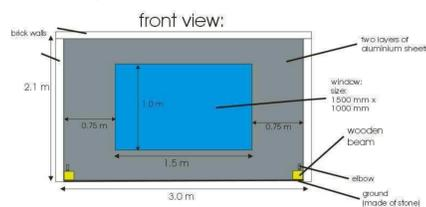
FIGURE 1: Wall construction and dimensions to test both standard and low emissivity window types.
