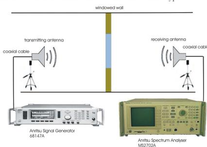
FIGURE 2: Experimental test set-up for both window types using X-band horn antennas.
