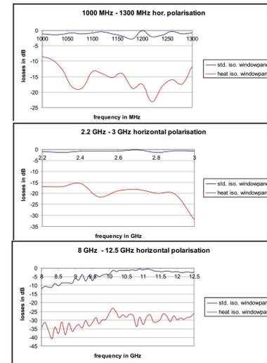
FIGURE 3: Relative propagation performances of both standard and low emissivity window types.
