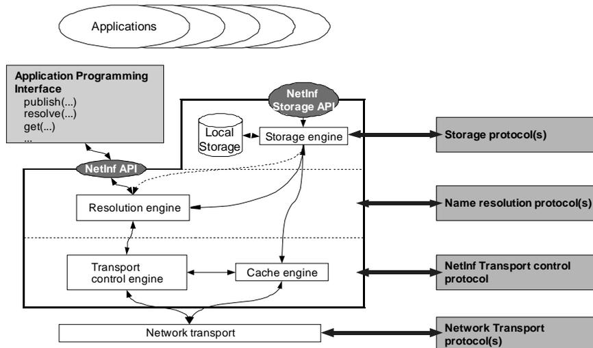
Figure 2: NetInf High-level Architecture.
