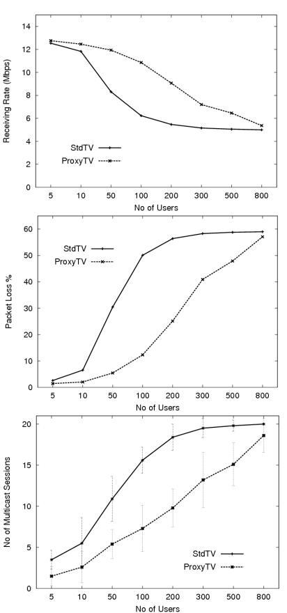
**Figure 5.** Statistical performances with and without *ProxyTV* (100 Mbps link bandwidth). a. (top) Receiving rate; b. (middle) Packet loss rate; c. (bottom) Multicast sessions.
