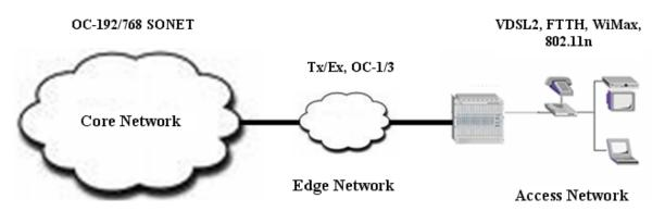
Figure 1. Existence of an edge network bottleneck.
