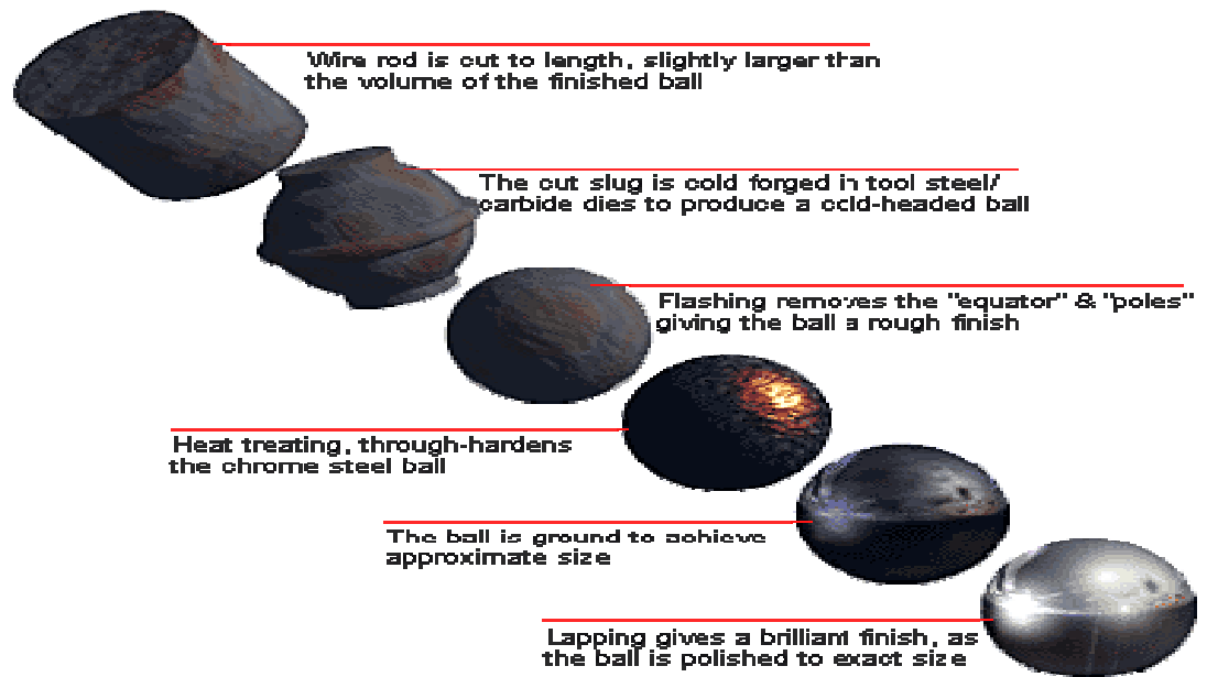
Fig. 2 Ball bearing appearance at stages of manufacture [52]
