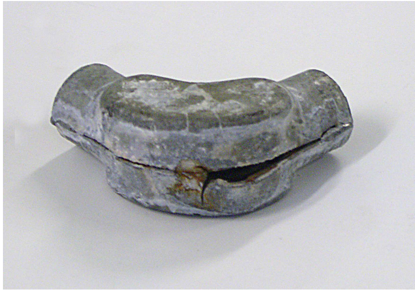
Fig. 21: Damage caused to steel elbow piece by samples
