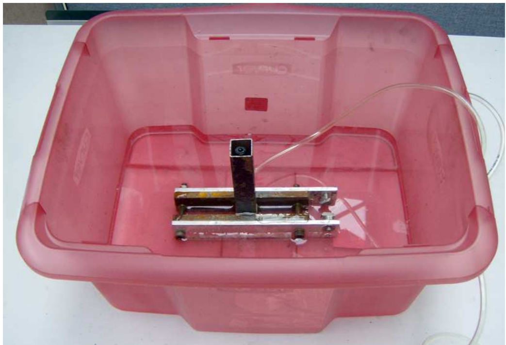
Fig. 37: Mock-up piezo chamber in a water bath
