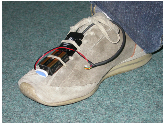
Figure 4.2: A foot mounted inertial platform for pedestrian navigation used at DLR.
