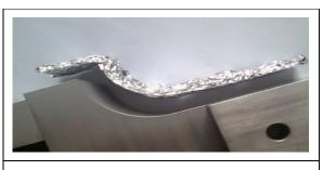
Fig. 189 Thermal shield made from crumpled kitchen foil.
