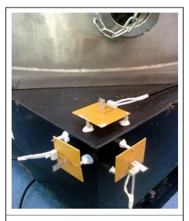
Fig. 195 MSIUSA<sup>™</sup> piezo film vibration sensors orientated orthogonal to each other on the granite block.
