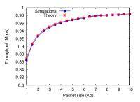
Fig. 2. Throughput analysis: 20 nodes, 1 Mbps rate, initial back-off windows equals 32, maximum back-off extension equals 5
