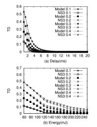
Fig. 8 Evaluation: IEEE 802.11b, 12 nodes, 1Kb/packet, 11Mbps/channel, Load 0.4: (a) Packet delay and (b) transmission energy TD.
