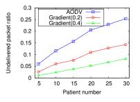
Fig. 13. Gradient based routing evaluation - ratio of packets undelivered to the gateways
