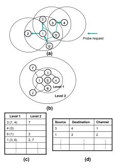
Fig. 3. (a) Node 5 sensing neighbours probe request, (b) virtual topology, (c) virtual topology table by node 5, and (d) channel table of node 5
