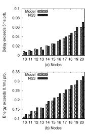
Fig. 10 Evaluation: IEEE 802.11b, from 10 to 20 nodes, 1Kb/packet, 11Mbps/channel, overall load varies from 0.1 to 0.2: (a) packet delay exceeds 5ms and (b) transmission energy exceeds 0.1mJ
