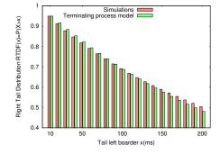
Fig. 4. Model evaluation packet delay right tail distribution. 30 Nodes
