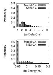
Fig. 7 Evaluation: IEEE 802.11b, 12 nodes, 1Kb/packet, 11Mbps/channel, Load 0.4: (a) Packet delay and (b) transmission energy distributions.
