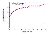
Fig. 3. Cooperation overhead analysis: 20 nodes, 1 Mbps rate, initial back-off windows equals 32, maximum back-off extension equals 5, 0.15s coordination delay
