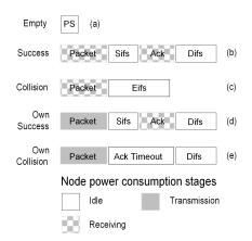
Fig. 1 Packet structure for different event types: IEEE 802.11 CSMA/CA Basic access scheme.
