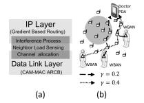
Fig. 8. Adaptive routing solution: (a) cross-layered integrated solution, (b) routing around high network load regions with different priority.
