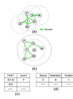
Fig. 4. (a) Node 5 sensing neighbours probe request, (b) virtual topology, (c) virtual topology table by node 5, and (d) channel table of node 5
