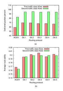
Fig. 8. Simulation results: (a) Percentage of delivered packets, (b) Average node ability along path
