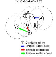
Fig. 3. Redundant channel blocking in CAM-MAC protocol
