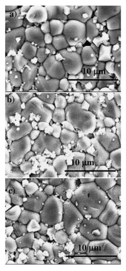
$\it a$  prepared from nano-ZnO;  $\it b$  prepared from micrometre-ZnO;  $\it c$  commercial varistor
