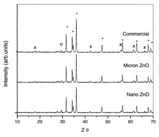
3 XRD pattern of sintered (1050°C) varistor samples (\* ZnO; x Zn<sub>7</sub>Sb<sub>2</sub>O<sub>12</sub>; o Bi<sub>2</sub>O<sub>3</sub>)
