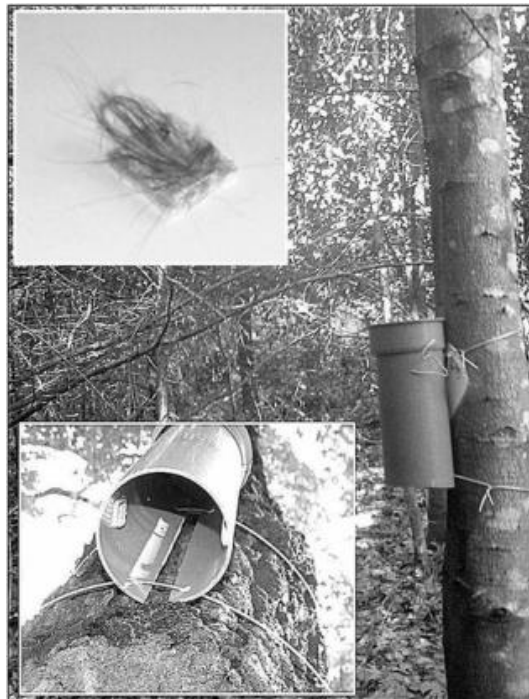
Fig 1.30: Hair-tube design used in Mullins et al. (2010) to collect pine marten hair non-invasively. The top inset is a hair-patch containing pine marten hair. The lower inset is a view into the hair-tube showing the placement of the sticky patch.
