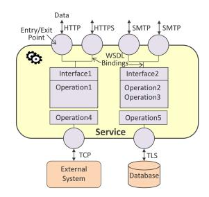
Figure 5.2: Example Service Entry/Exit Points
