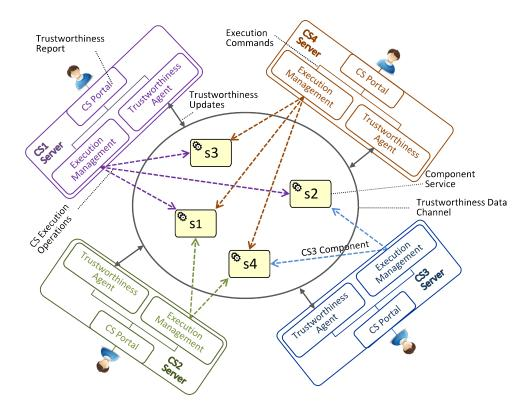
Figure 6.1: Trustworthiness Data Exchange Framework
