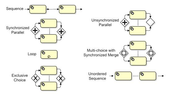
Figure 2.1: Common Service Composition Constructs
