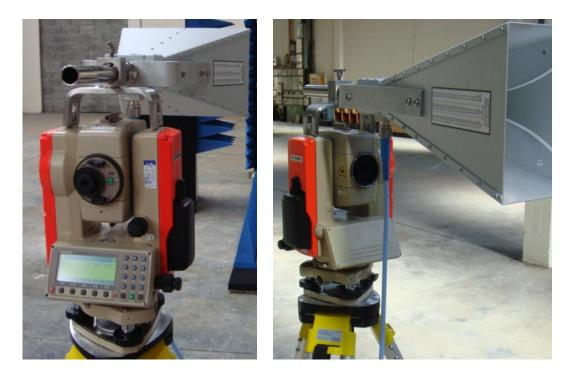
Figure 3-3 Modified Pentax Total Station for antenna mounting
