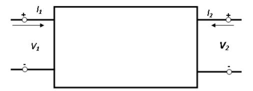
Figure 4-3 Two-port transmission network
