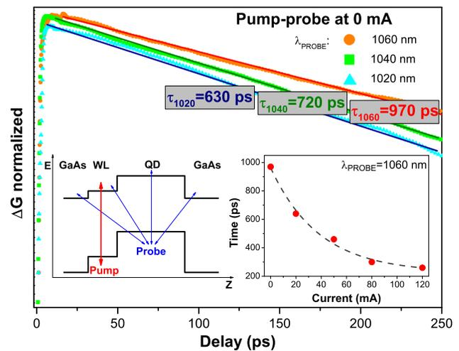
FIG. 2. Normalized change of the gain at different probe wavelengths at 0 mA bias. Inset: schematic of states pumped and probed during a single measurement and corresponding decay constant as a function of the bias current.
