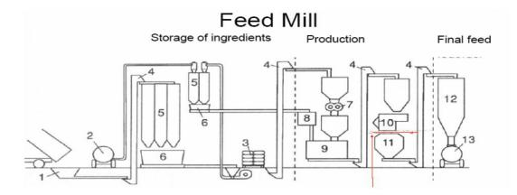
1. Intake pit for trucks, 2. Pneumatic intake, 3.Intake pit for bags, 4. Elevators, 5. Storage bins, 6. Scales, 7. Mill, 8. Pre-bin for premixes, vitamins etc., 9. Mixer, 10. Conditioner and pellet press, 11. Pellet cooler, 12. Storage bin for compound feedingstuffs, 13. Bulk truck
