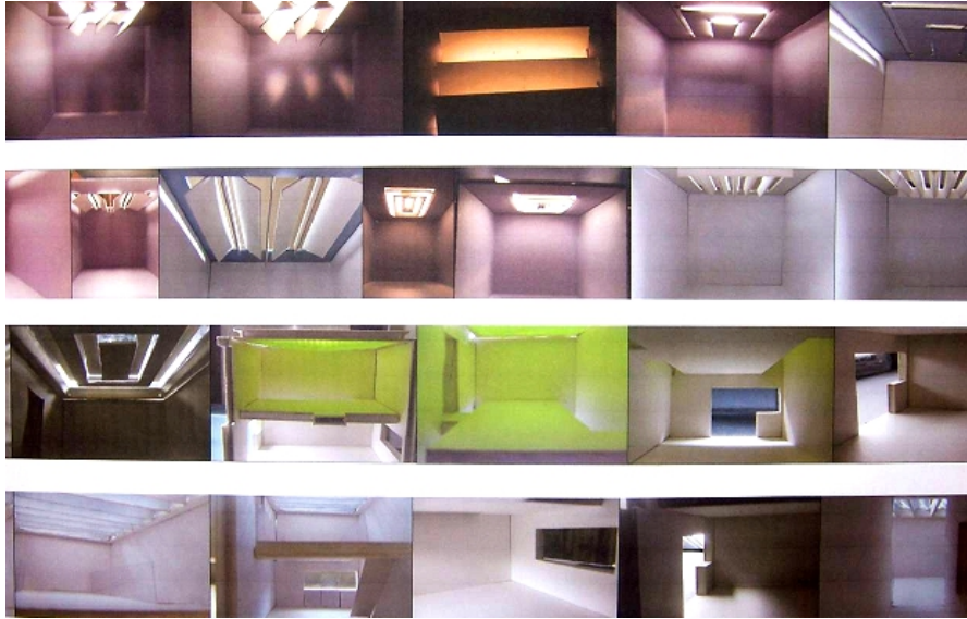
Daylight study by Sean Kehoe, exploring light distributors in the ceiling and considering the "colours" of light
