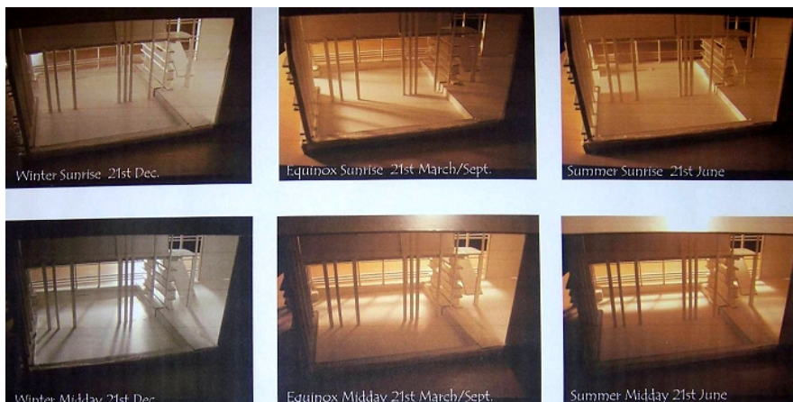
Daylight study by Gary Nash: Simulating daylight and its different qualities throughout the seasons
