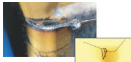
Figure 2-12: Notch wear – Sandvik
