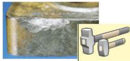
Figure 2-15: Edge chipping/breakage – Sandvik
