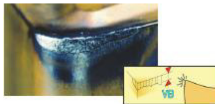
Figure 2-9: Flank Wear – Sandvik
