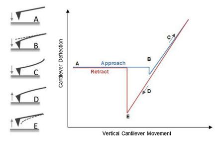
Fig. 4. Cantilever deflection recorded in force distance curve. Cantilever deflection vs. cantilever movement in one approach and withdraw cycle. The cantilever deflection is then converted into force to result in a force curve, showing the point of snap-on, B, and the point of snap-off, E.
