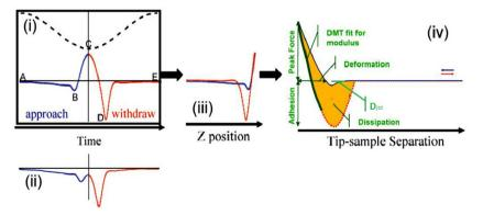
**Fig. 2.** Force distance curve acquisition and conversion. (a) Plot of force and z-piezo position as a function of time, including (B) snap-on, (C) peak force, (D) snap-off, (b) plot of force vs. time, (c) force curve consisting of plotting force vs. z-piezo position, (d) plot force vs. separation and information given by the plot. Reprinted with permission from Bruker Nano Surfaces Division, Tucson, AZ, USA.
