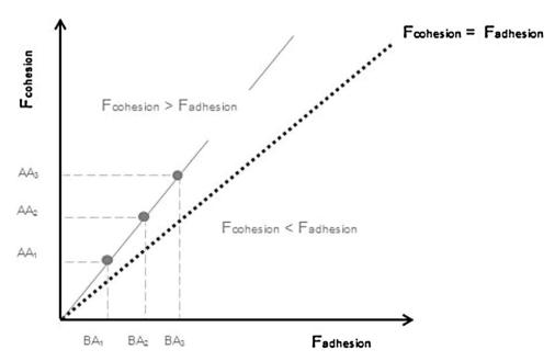
**Fig. 7.** CAB plot of adhesive against cohesive forces. Three different colloid probes of material A have been used to measure the adhesion between substrate B and A (BA<sub>1</sub>, BA<sub>2</sub>, BA<sub>3</sub>) and the cohesion between substrate A and A (AA<sub>1</sub>, AA<sub>2</sub>, AA<sub>3</sub>). The cohesive forces exceed the adhesive forces.
