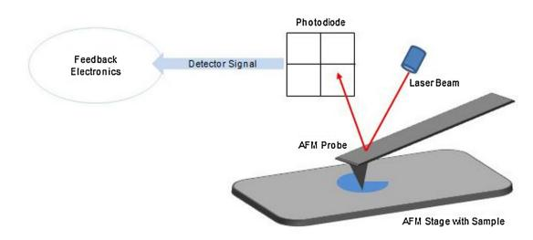
**Fig. 1.** Schematic overview of AFM measurements. The sample is scanned by an AFM probe onto which a laser beam is directed and reflected onto a four-quadrant photodiode. The signal from the photodiode is then evaluated by the feedback controller. Piezoelectric elements are included in the scan head or the AFM stage to ensure precise motion in the nanoscale.
