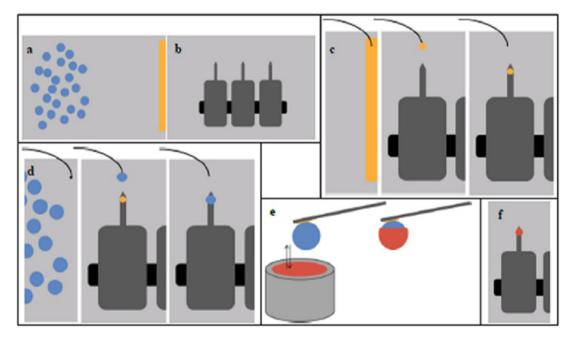
**Fig. 3.** Colloidal probe AFM. (a) Preparation of glue and glass microspheres on a silicon wafer, (b) preparation of tipless cantilevers on a silicon wafer, (c) dropping glue onto the free end of a cantilever with a needle, (d) moving glass microsphere to the cantilever with a needle, (e) dipping glass microsphere into a dispersion for coating (optional) and (f) coated glass microsphere glued to the cantilever.
