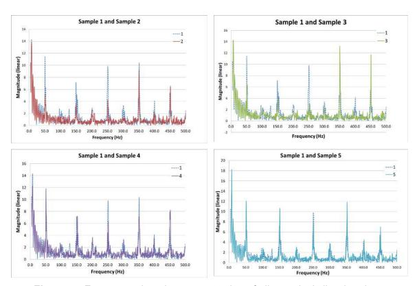
Figure 57 Frequency domain representation of all samples' vibration data
