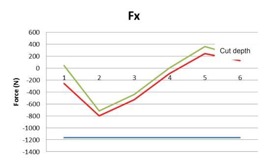
Figure 60 Sensor X-axes force for depths 1-6mm
