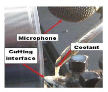
Figure 5 Microphone configuration
