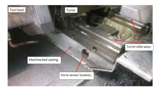
Figure 23 Force sensor location in relation to slideways and turret
