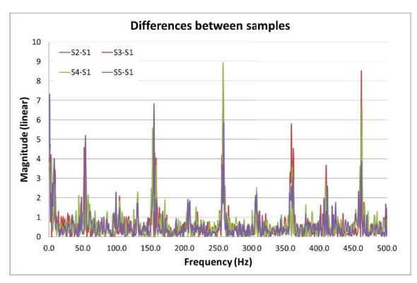
Figure 58 Frequency domain differences between samples' vibration data
