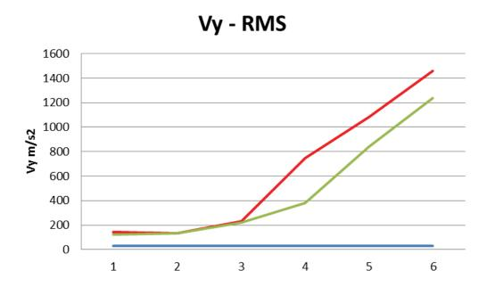
Figure 64 Sensor Y-axes vibration for depths 1-6mm
