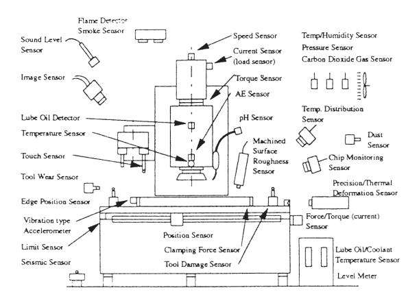
Figure 1 Illustration showing the various researched sensor systems
