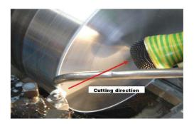
Figure 6 Detail of Insert/workpiece
