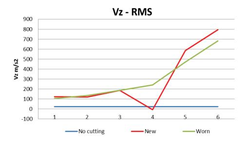
Figure 65 Sensor Z-axes vibration for depths 1-6mm
