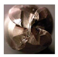
Figure 40 Worn tool- front view 50X
