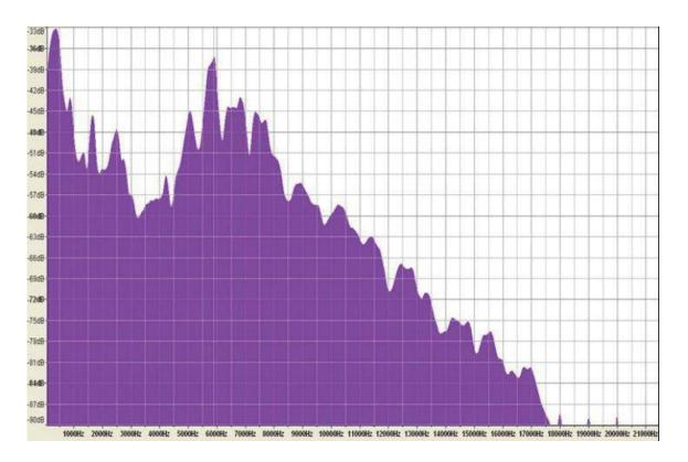
Figure 9 Frequency domain representation of a Harrison lathe audio signal
