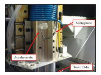
Figure 12 Sensor locations on machine spindle
