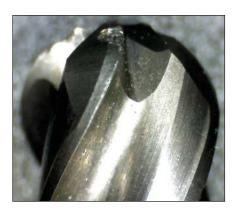
Figure 42 Worn tool- side view 50X
