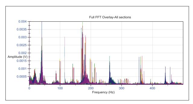
Figure 46 Full FFT spectrum overlay of all sections (vibration sensor 1).
