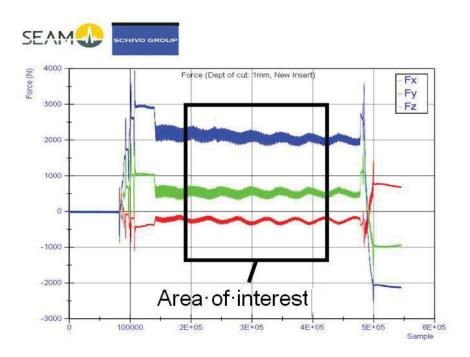
Figure 59 Force sensor results for each axis, 1mm cut, and area of interest
