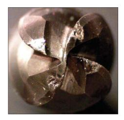
Figure 16 Photos of new and exhausted ballnose cutter X50 Magnification
