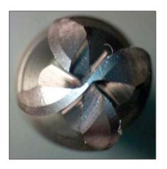
Figure 39 New tool- front view 50X
