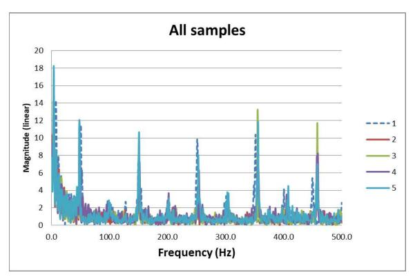
Figure 56 Frequency domain representation of all samples' vibration data
