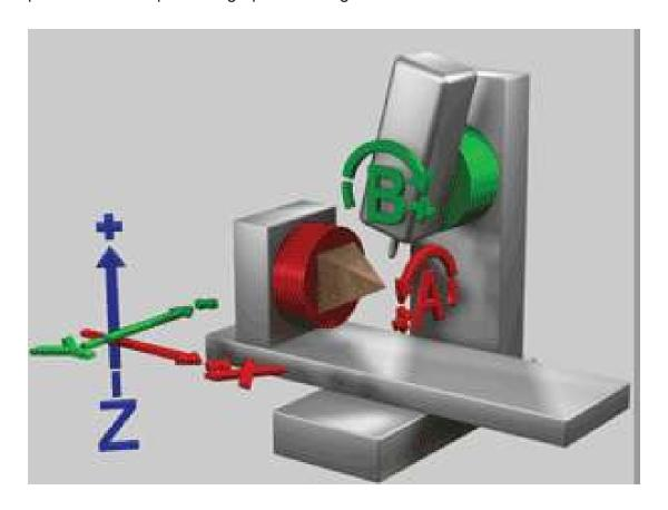
Figure 70 Illustration of axes in CNC turning
