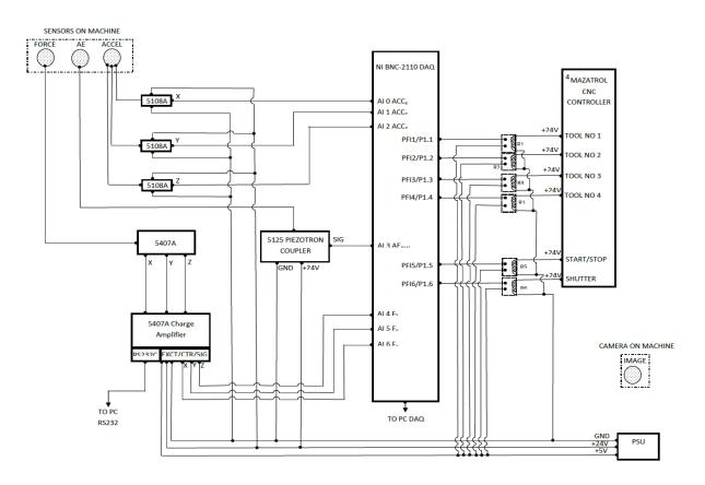
Figure 20 Monitoring system circuit diagram
