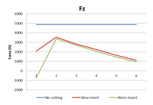
Figure 62 Sensor Z-axes force for depths 1-6mm
