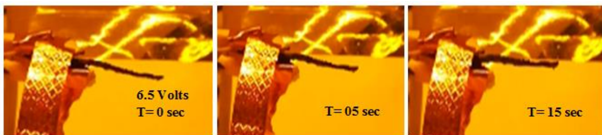
Figure 8.18 Bending capabilities of sulfonated SEBS with scCO 2
