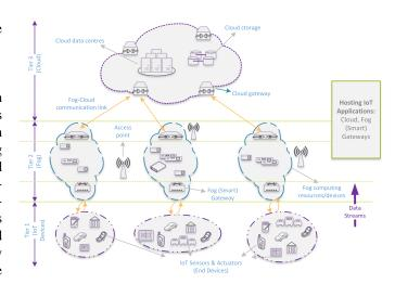
Fig. 1. Fog-Cloud Architecture (Distributed Data Processing) in standardized IoT architecture
