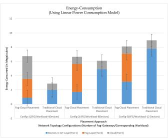
Fig. 6. Variation of energy consumption in both the placement approaches— Creating a balance between energy consumption at high (Cloud data centres) and low (Fog layer) cost sites by spreading computing across the network
