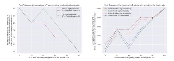
(a) Plot representing number of the times the user (b) Plot representing average service delivery time access query was served in three experimental by the system for user access queries during fault tolerance experimentation.
