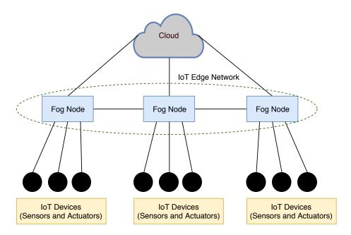
Fig. 5.2 Tree Topology in Fog Enabled IoT Deployments [14].
