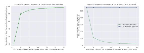
(a) Effect of changing data processing frequency (b) Effect of changing data processing frequency at fog node VMs and corresponding % reduc- at fog node VMs and corresponding reduction in tion in data transfer to cloud using fog based dis- data transfer to cloud using fog based distributed tributed data analytics approach compared to tra- data analytics approach compared to traditional cloud centric approach.
