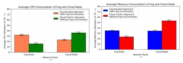
(a) Average CPU utilization at fog and cloud node (b) Average Memory utilization at fog and cloud node
