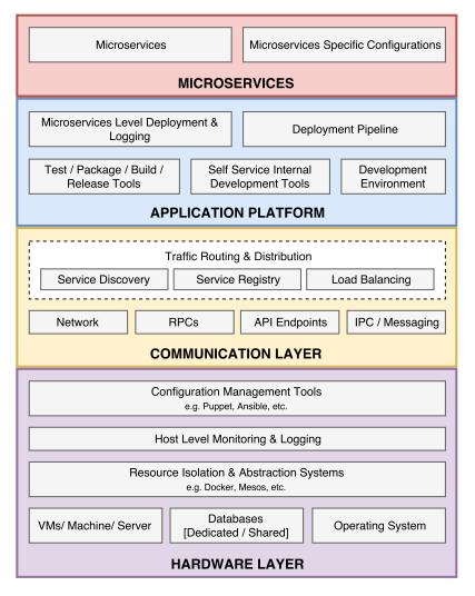
Fig. 2.9 The four-layer model of microservice architecture- A comprehensive breakdown of what lies in the four layered microservices architecture [75], [7]. API, application programming interface; IPC, interprocess communication; RPC, remote procedure call
