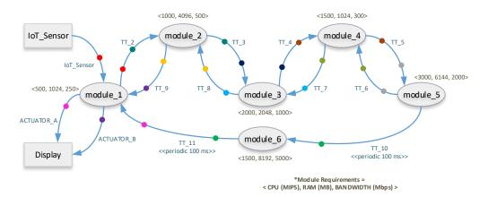
Fig. 4.2 Directed Acyclic Graph (DAG) of the application deployed, with relevant tuples indicating the values used for simulation of the algorithm. The number of modules as well as sensors/actuators are synchronous to the needs of a typical IoT application, and may vary as per the use case and application size; the modules can be conveniently linked to various logics to convey the various stages of application processing, as are the ones conveyed by the color pair encoding here [12].
