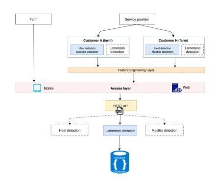
Fig. 3.9 Proposed microservices based application design and flow for integration of services from different service providers [6], [9].
