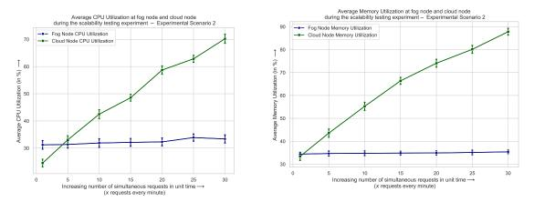
(a) Plot representing average CPU utilization at (b) Plot representing average memory utilization fog and cloud node during the scalability testing at fog and cloud node during the scalability testing experiment in scenario 2.
