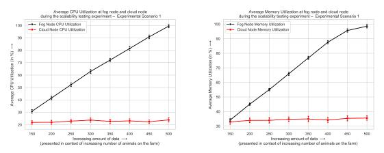
(a) Plot representing average CPU utilization at (b) Plot representing average memory utilization fog and cloud node during the scalability testing at fog and cloud node during the scalability testing experiment in scenario 1.
