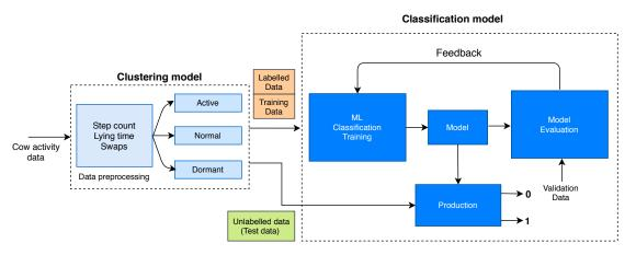
Fig. 3.32 Designed hybrid machine learning model for early lameness detection consisting of activity-based threshold clustering followed by the classification model.
