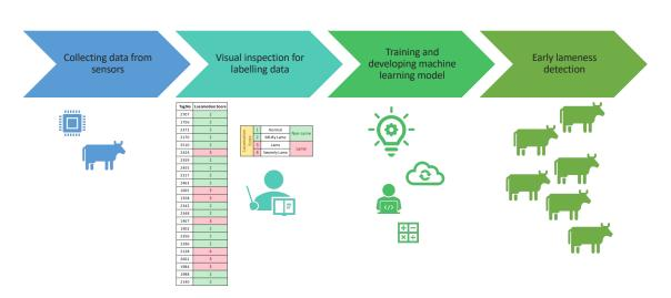
Fig. 3.31 A diagrammatic representation of the end-to-end pipeline of the developed solution illustrating: 1) data collection from sensors, 2) observation of animals by an animal expert to give locomotion score, 3) translating the human observer's expertise into a machine learning based system leading to early detection of lameness in cattle.
