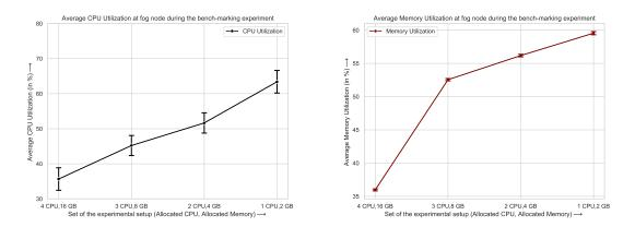
(a) Plot representing increase in average CPU uti- (b) Plot representing increase in average Memory lization at fog node with decreasing quantity of utilization at fog node with decreasing amount of allocated CPU.
