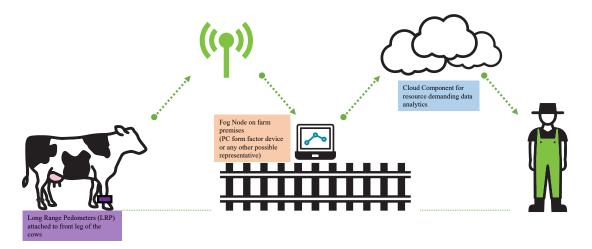
Fig. 3.1 A high-level diagrammatic representation of the system workflow, and different components of the developed IoT solution [8].
