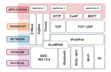
Fig. 2.7 Overview of Communication Protocols with respect to OSI model [71]
