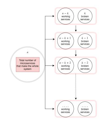
Fig. A.3 Diagrammatic representation of services getting broken and getting back into the pool of working service sequentially one after the another.
