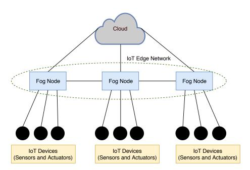
Fig. 2.6 Tree Topology in Fog Enabled IoT Deployments [14].
