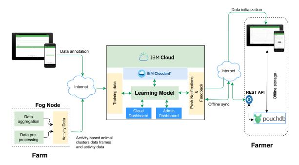
Fig. 3.8 Mobile application developed specifically considering the needs of the farmer, including an offline first strategy. The figure presents data and notification flow in the developed mobile application [9].
