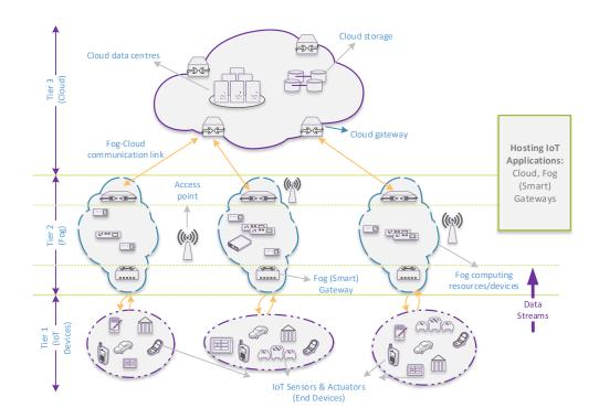
Fig. 4.1 Three tier IoT-fog-Cloud architecture illustrating distributed data processing [12].
