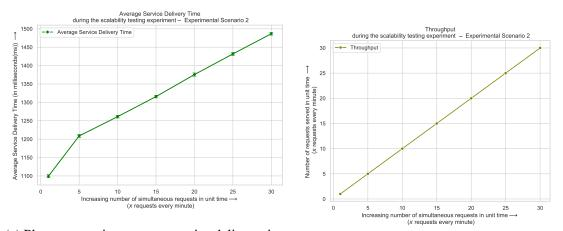
(a) Plot representing average service delivery time during the scalability testing experiment in scenario 2.(b) Plot representing throughput during the scalability testing experiment in scenario 2.
