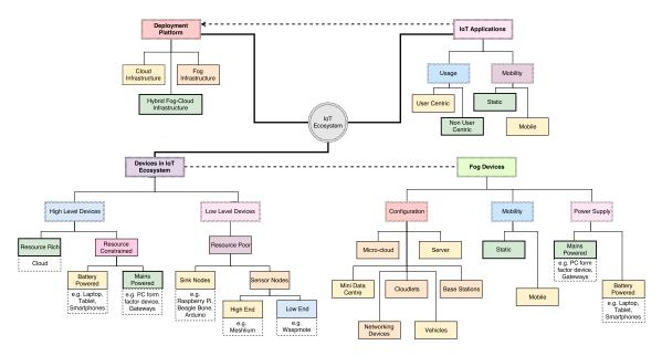
Fig. 2.5 Visual representation of IoT Ecosystem illustrating IoT devices, available deployment platforms and type of IoT applications [7].
