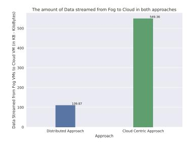
Fig. 5.10 Reduction in amount of data being streamed from fog VMs to cloud VM in fog based distributed approach.
