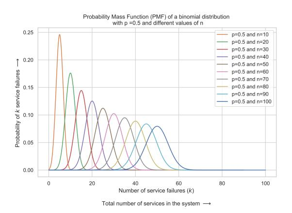
Fig. A.1 Plot presenting probability mass function(pmf) of binomial distribution with p=0.5 and different values of n. We map this pmf with the number of service failures and probability of such service failures in the system.
