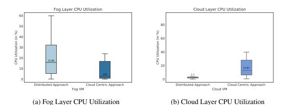
Fig. 5.8 CPU utilization visualized for both the distributed and cloud centric approach.
