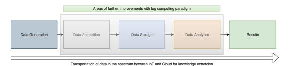
Fig. 2.13 A comprehensive view of data collection pipeline and highlighting the areas with a scope of improvement by incorporation of the fog computing paradigm.
