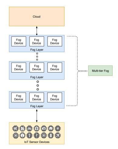
Fig. 2.4 Fog computing architecture representation as three tier IoT-fog-cloud architecture with multi-tier fog in a standardized IoT reference architecture model [41], [10], [12].
