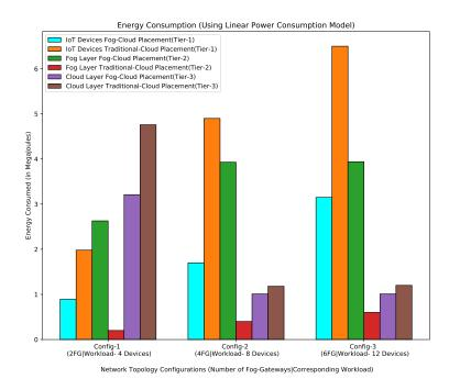
Fig. 4.6 Variation of energy consumption in both the placement approaches— Creating a balance between energy consumption in the cloud (at cloud data centres) and in fog layer (fog devices) by spreading computing across the network. The energy consumption in the cloud data center decreases when application modules are placed on fog devices using the proposed Fog-Cloud Placement approach compared to the Traditional-Cloud Placement strategy.
