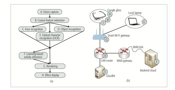
Fig. 2.11 Directed Acyclic Graph (DAG) of an application and its deployment onto the infrastructure [126], [127]. (a) DAG of a cognitive assistance application, (b) Deployment of this DAG onto the computing resources available in the infrastructure.
