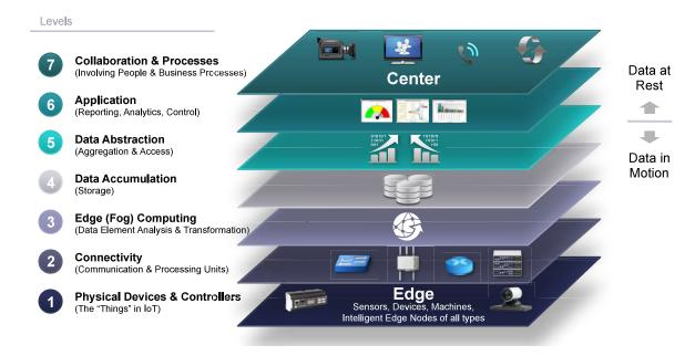
Fig. 2.3 The Cisco IoT Reference Model [29].
