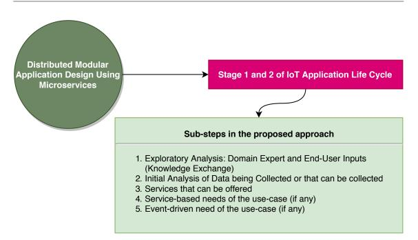
Fig. 3.4 The sub-steps of the proposed approach that need to be included in the stage 1 and 2 (plan and design) of the IoT application life cycle.
