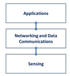
Fig. 2.1 Three Tier IoT Architecture by IEEE P2413 [24].
